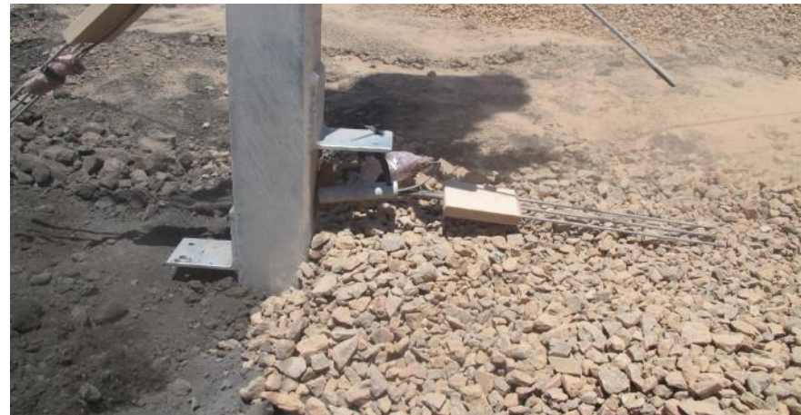
Sensors Buried In Tailings and Capillary Break
