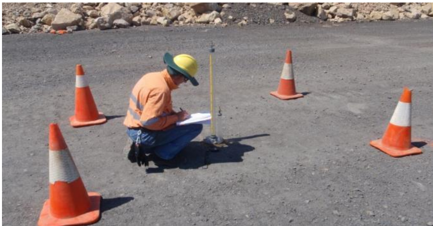
6. Quality Control RPL Permeability Testing
