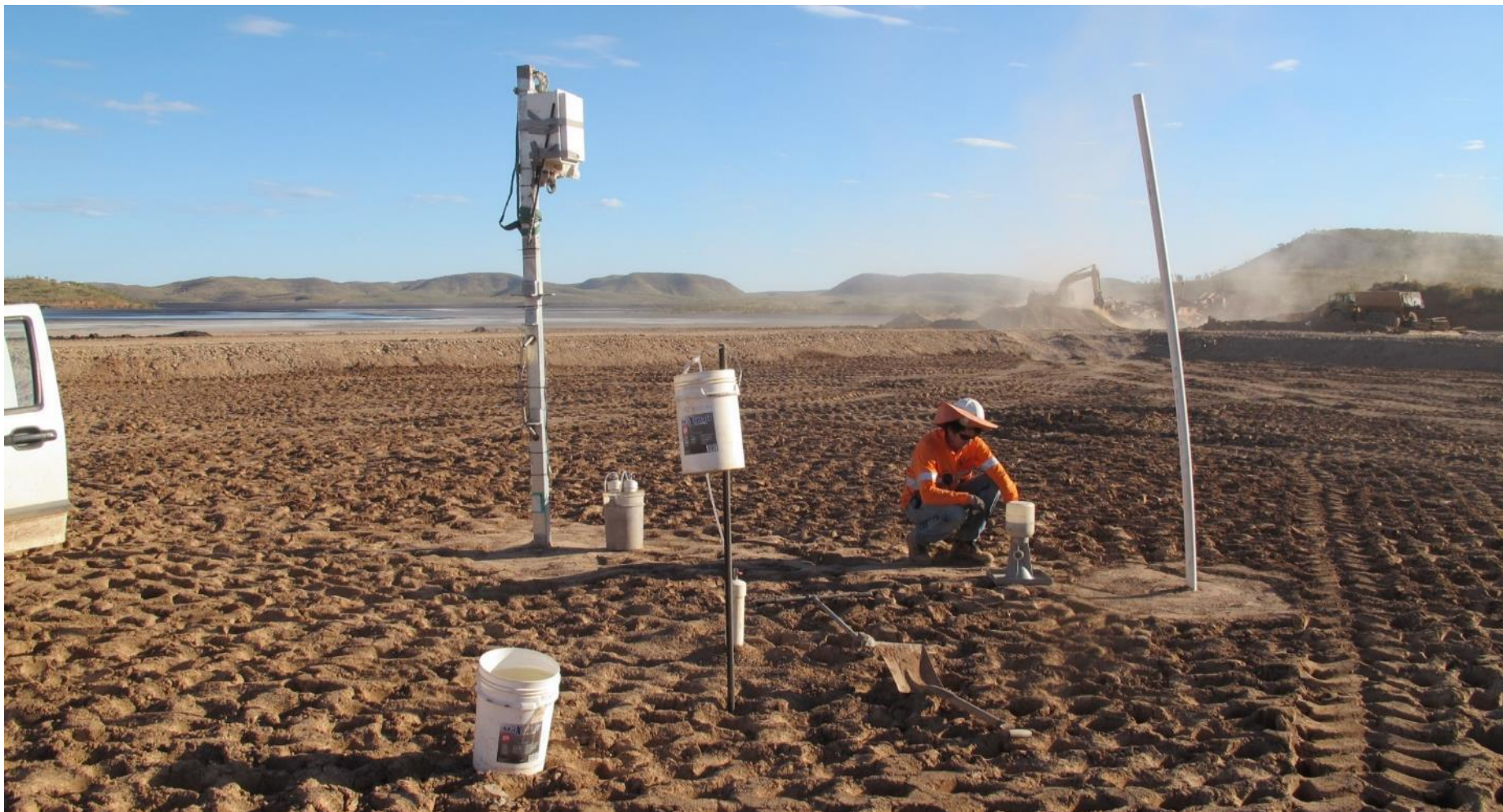
Permeability Testing of RPL
