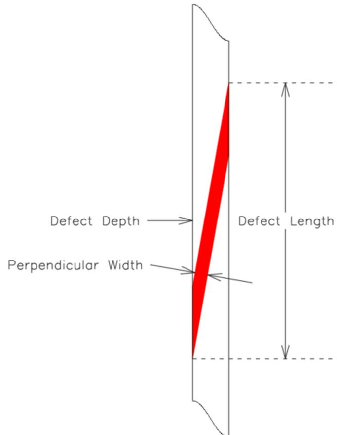
**Figure 4.9: Measuring Defect Depth, Defect Length and Perpendicular Width**
