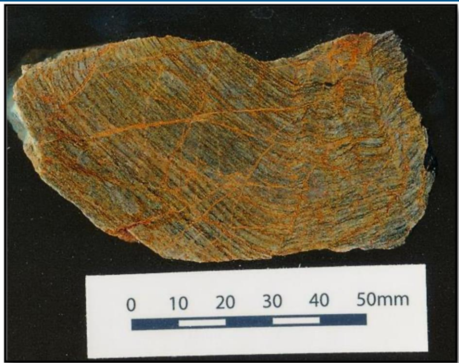
East Block – Arsenic-rich brittle fractures overprinting kink folds
