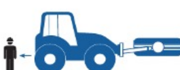
Operator not in the cab. Tyre handler rolls away, not chocked, handbrake fails, etc.
