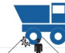
Air blast or projected tyre/wheel/rim component strikes fitter - within line-of-fire
