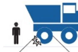
Air blast strikes fitter - outside line-of-fire but within 5 metres of tyre
