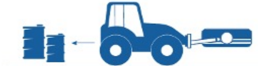
Operator not in the cab. Tyre handler rolls away, not chocked, handbrake fails, etc
