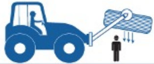
Fitter standing under the suspended load
