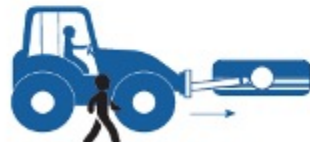
Walking perpendicular or at an angle within range of the tyre handler
