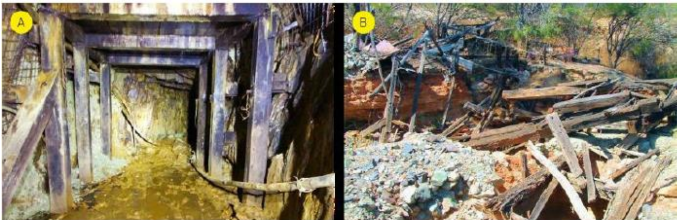
Abandoned mine workings, showing underground tunnel (A) and vertical shaft opening (B).
