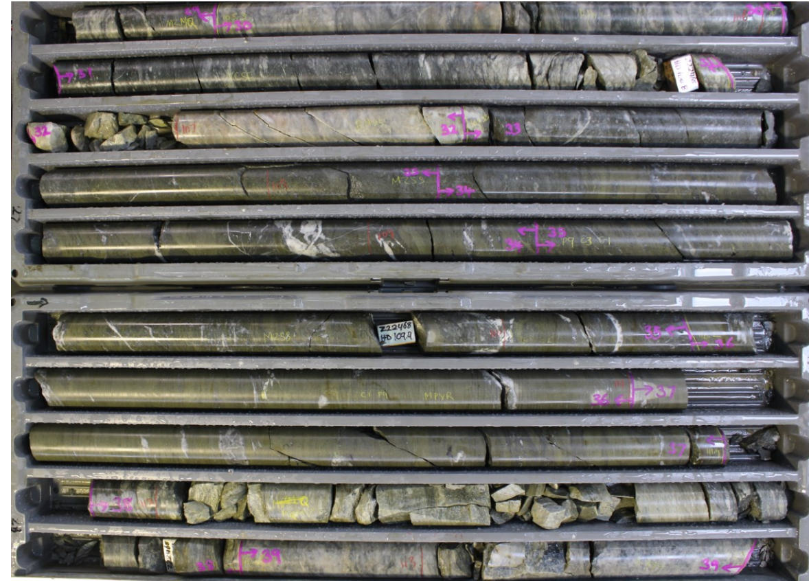
Z22468 Massive sulphide zone with late quartz-carbonate fill.
