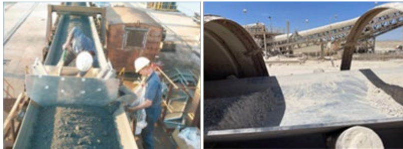
FIG 7 – Examples collection of the reference sample from a conveyor belt during a Bias Test.
