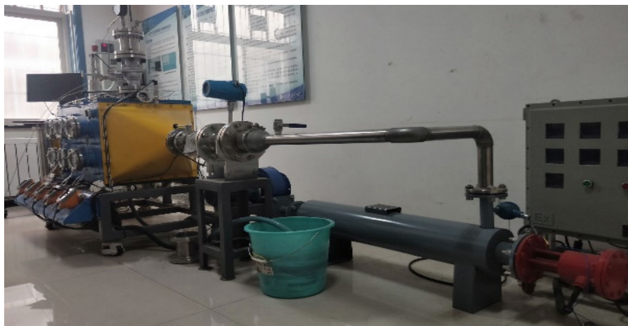
FIG 2 – Multi-factor influenced coal body gas desorption spraying experimental platform.
