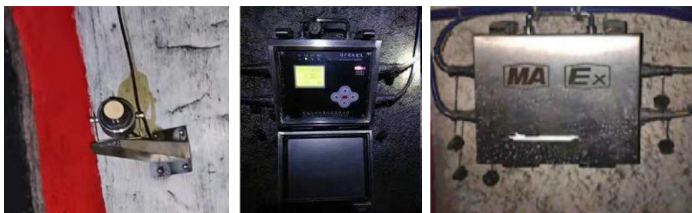
FIG 2 – Ultrasonic accurate wind measuring device.
