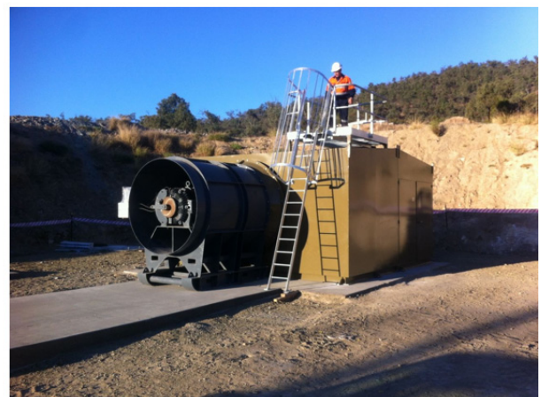
FIG 4 – 186 m Safescape Laddertube installed at Cracow Mine Site return airway.
