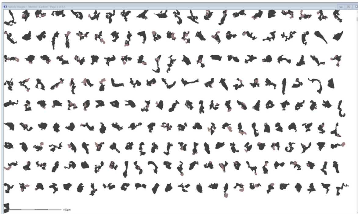
FIG 5 – Example of particles >50 Wt per cent carbon; black is carbon, light brown is chlorite.
