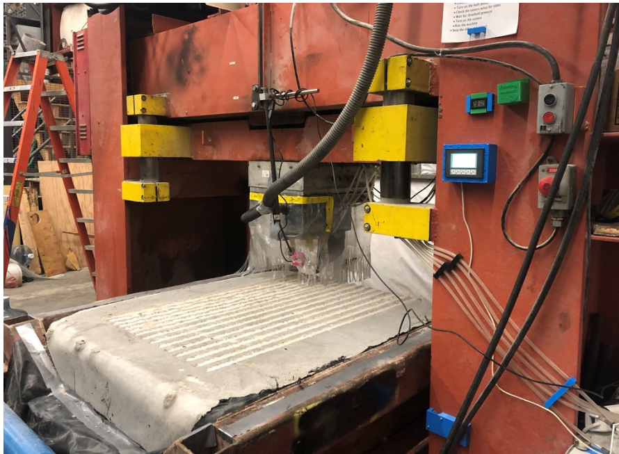
FIG 1 – The Linear Cutting Machine with the first set of conditioning cut lines on the surface of the concrete sample. The pick is encompassed by the dust curtain.
