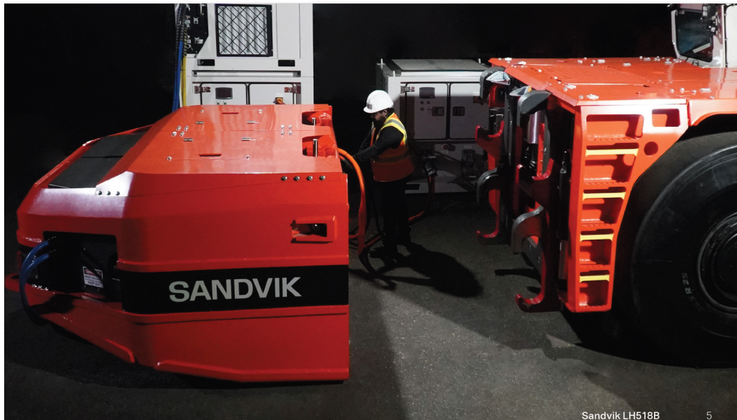
FIG 5 – The detachable battery module of an LH518B loader (Sandvik, 2021a).
