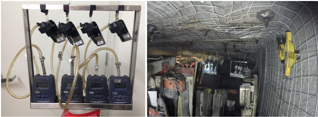
FIG 1 – (left) Respirable cyclone array on frame, (right) cyclone array mounted to continuous miner.
