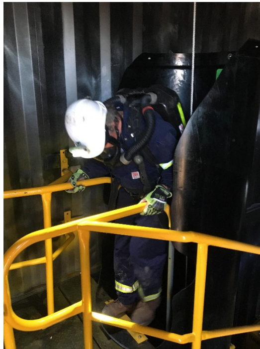
FIG 10 – Safescape Laddertube – carbon nanotube based polymer.
