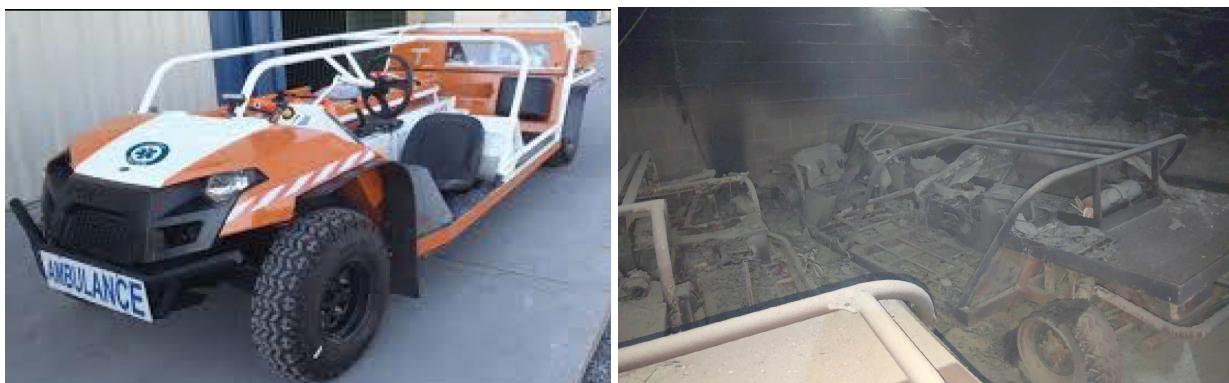
FIG 2 – BEV before and after – underground fire southern districts (Ontario Mine Rescue, 2021).
