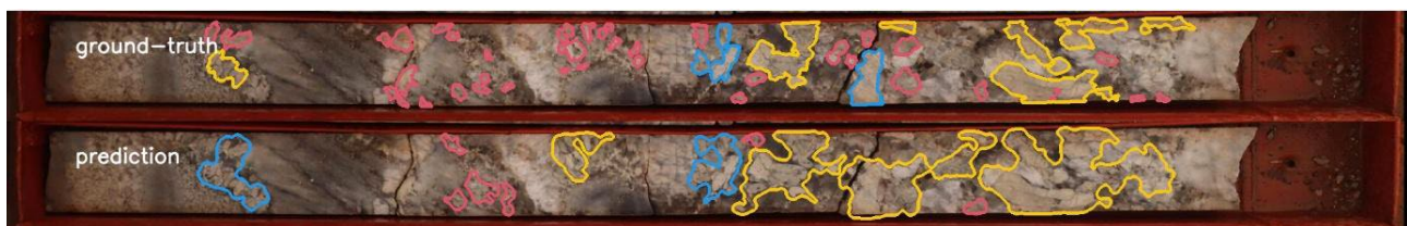
FIG 3 – Version 1 of the training results showed good detection of spodumene and differentiation from other minerals.
