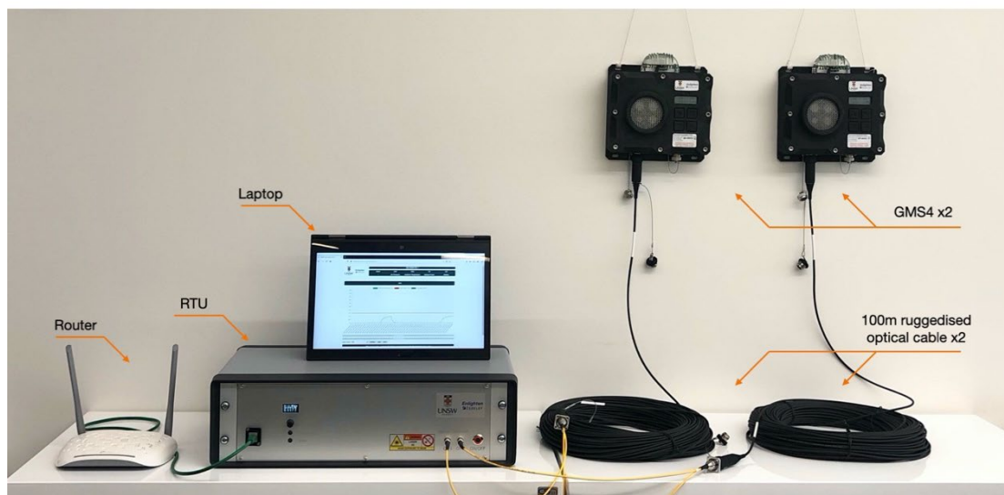
FIG 1 – Intrinsically safe, optically powered gas monitoring system. This exact system was deployed on December 17, 2020 at the BMA-operated mine of Broadmeadow.
