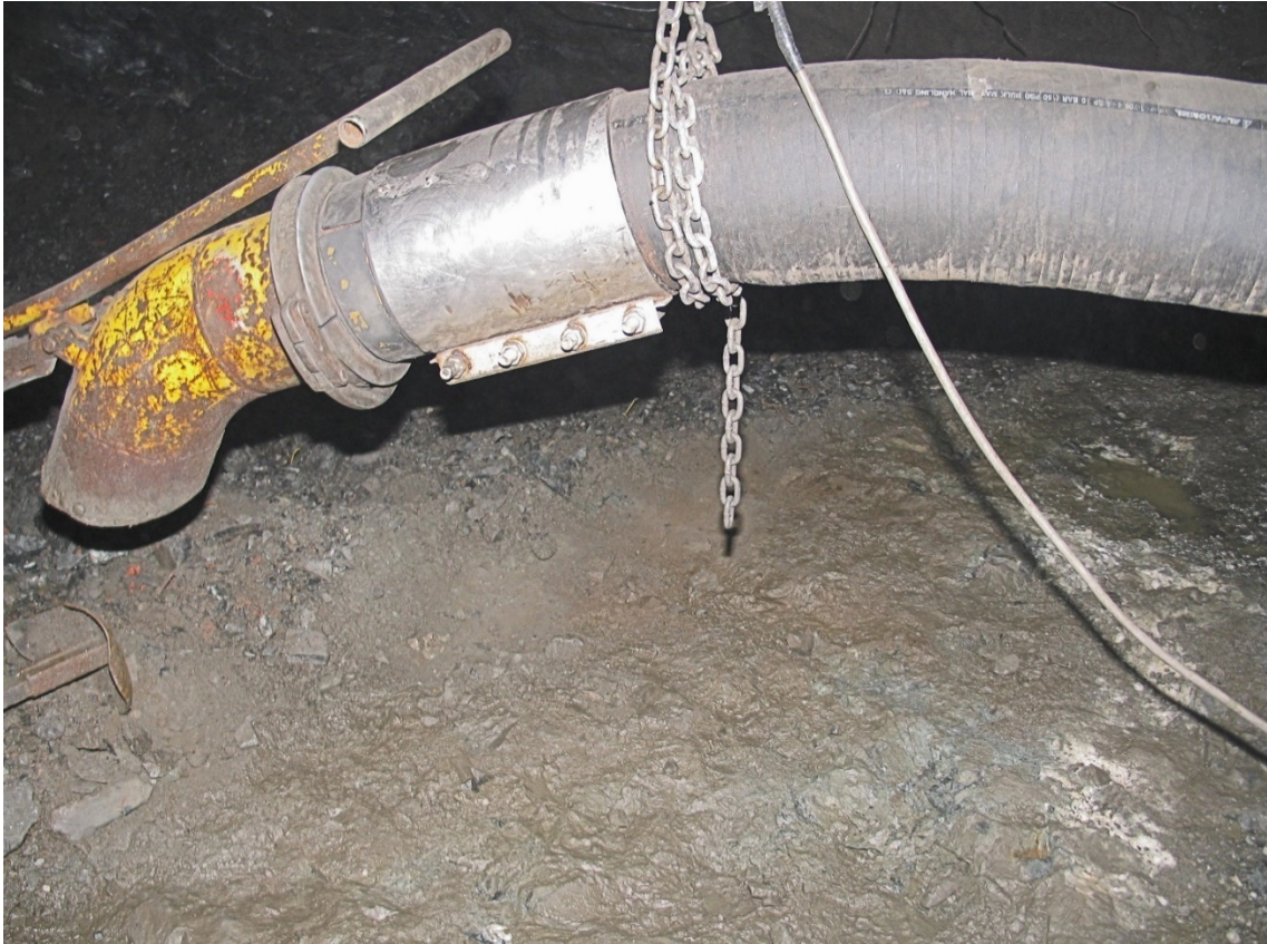
FIG 2 – Approximately ~0.35 m thick broken ore left behind on ore drive floor on the nickel mine located near Kambalda in WA – before and after vacuuming. Suction hose diameter 200 mm.
