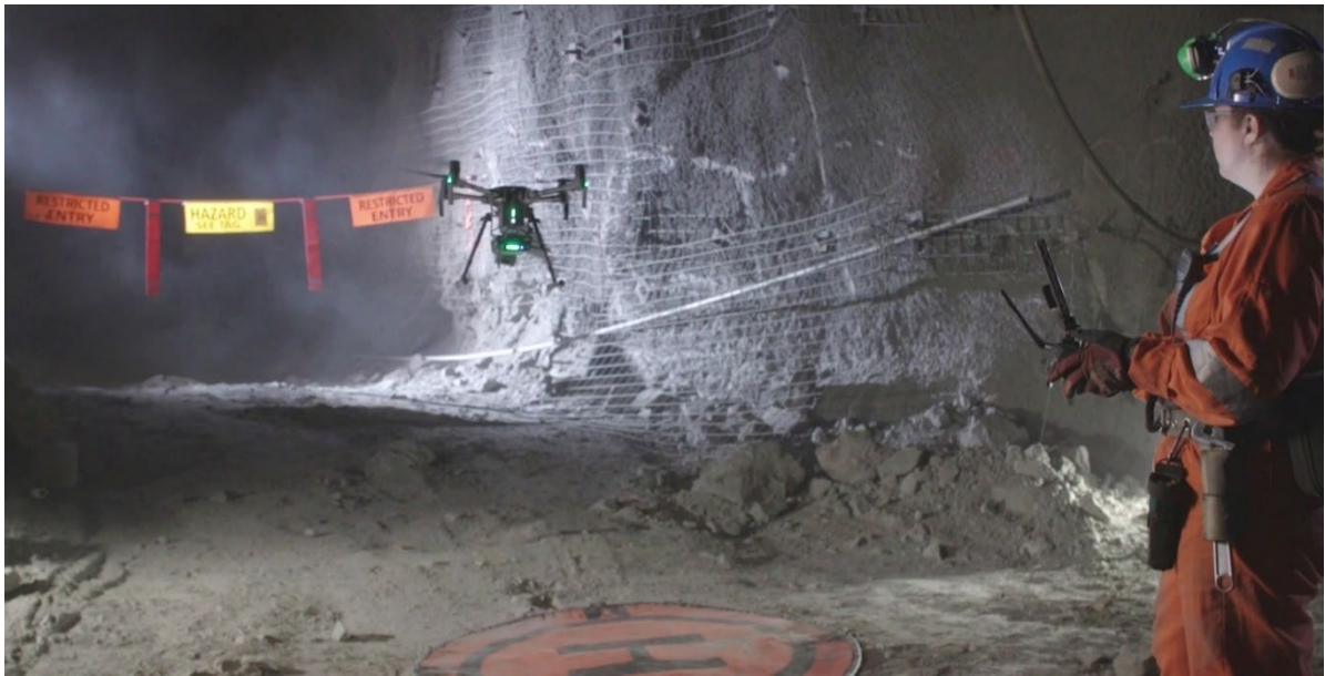
FIG 2 – Glencore’s Kidd Operations, an ultra-deep base metal mine located in Ontario, Canada, deploys Hovermap to remotely inspect stopes and drives throughout the mine.
