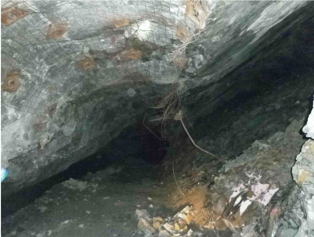
FIG 1 – Development drive and low-angle stope floor after mucking by scraper. Remaining fines material in both the drive and stope floor contains liberated gold.
