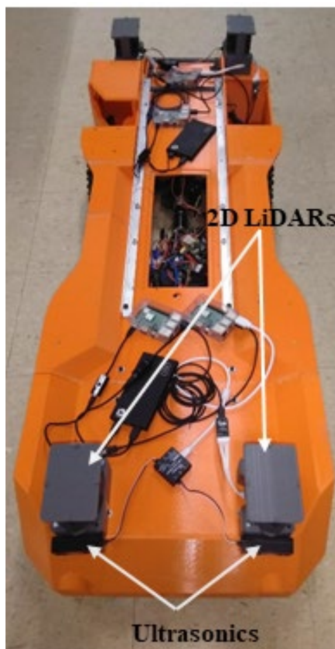
FIG 4 – Prototype equipped with LiDAR units and ultrasonic sensors.
