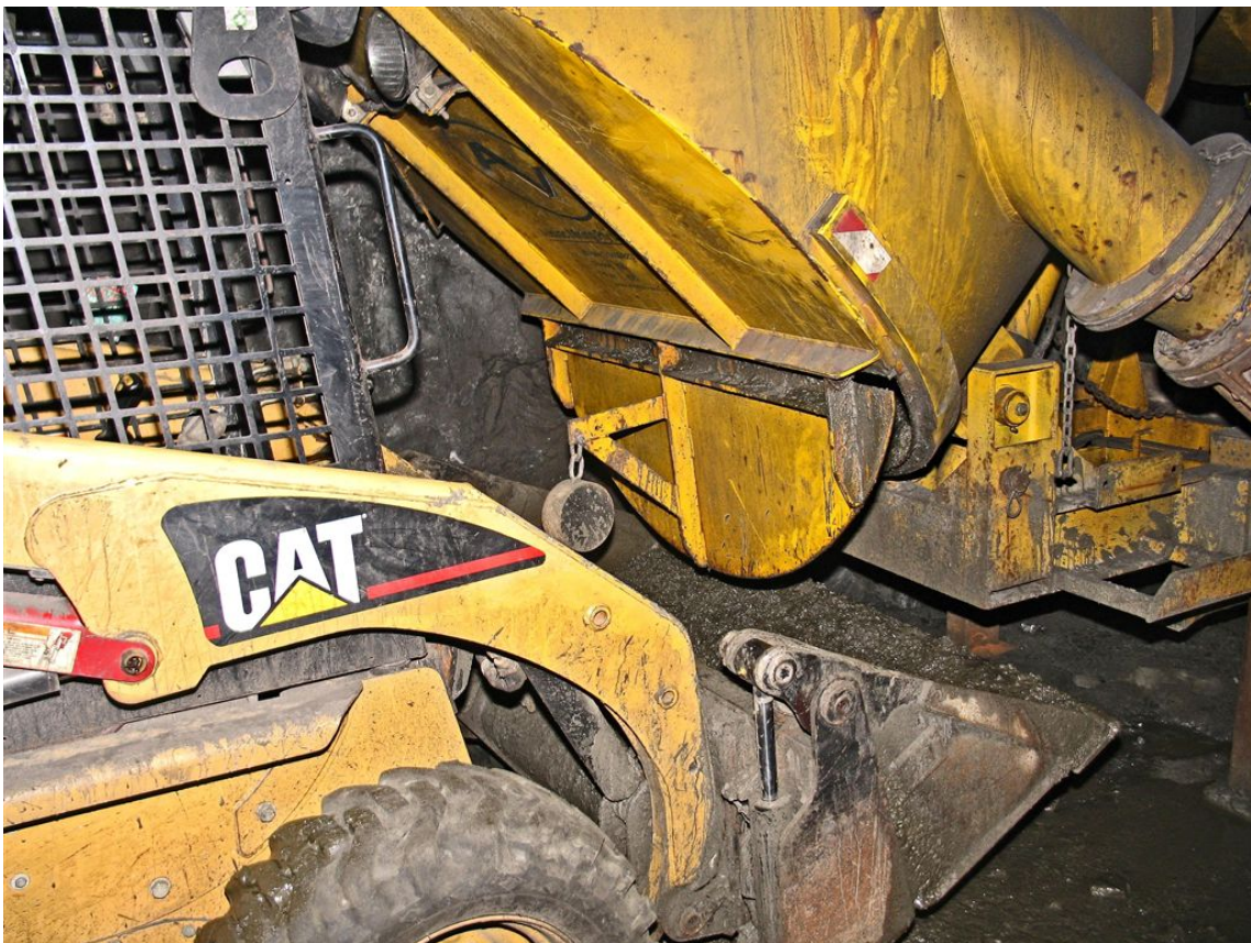
FIG 3 – Discharge from the bin into the Bobcat/Cat Skid Steer loader – Nickel Mine near Kambalda, WA.
