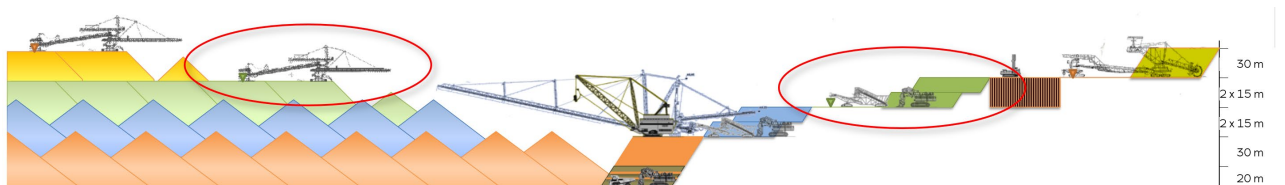
FIG 6 – Cross-section of a typical opencast strip mine with different mining systems.
