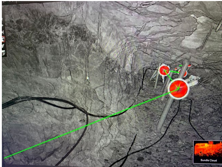
FIG 6 – A grey scale pointcloud of the reef drive exposing VCR reef.
