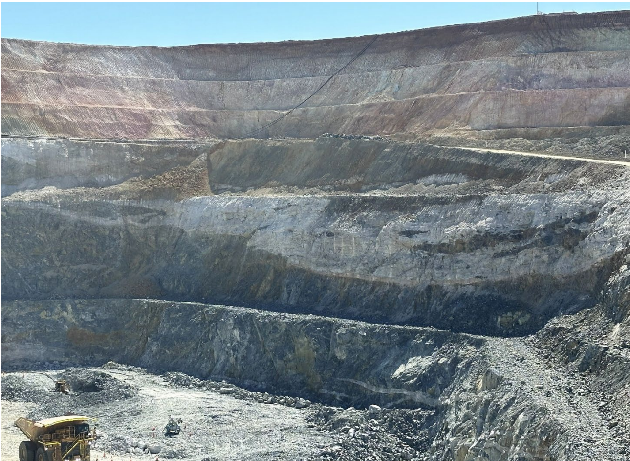
FIG 1 – Geology exposed at Mt Holland lithium mine. Pale shallow dipping unit in second lowest bench is pegmatite ore. Note local offsets, mafic xenoliths, and lateral pinch outs.
