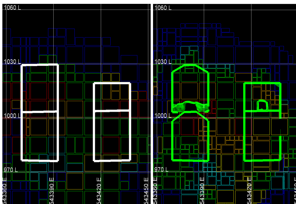
FIG 3 – In cross-section, example of 3D Budget design solids in against resource model (left) and 3D GCD against GC model (right).
