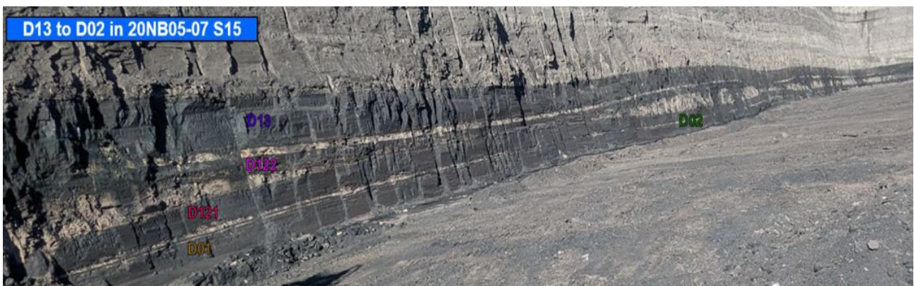
FIG 4 – Example of Z-splitting between the Dysart Seams, demonstrating rapid lateral change in seam splitting relationships.
