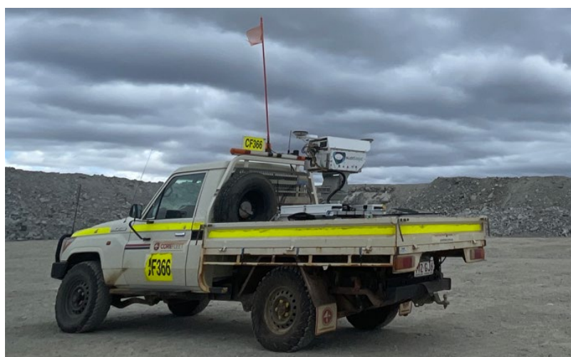
FIG 3 – OreSense® Ranger system hardware.
