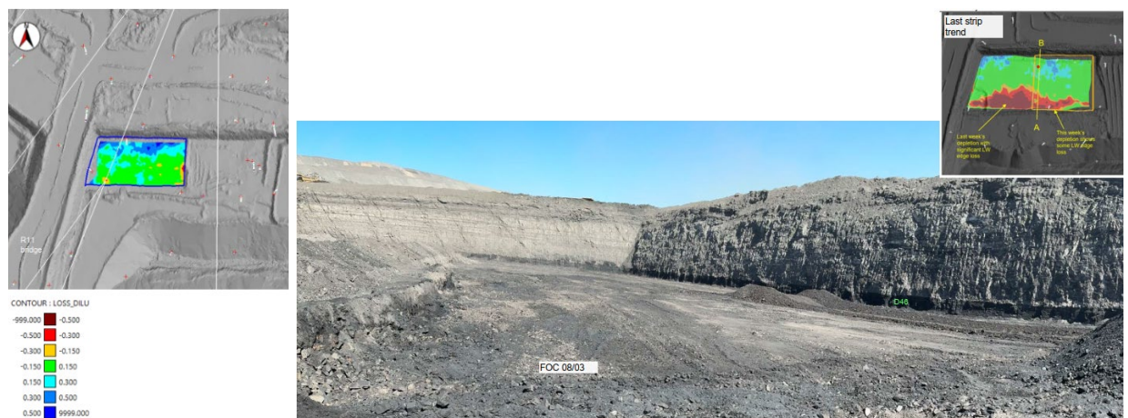
FIG 13 – Representative D46 (thin seam) shows very good compliance, but any differences with the mined thickness can be attributed to the irreducible error.
