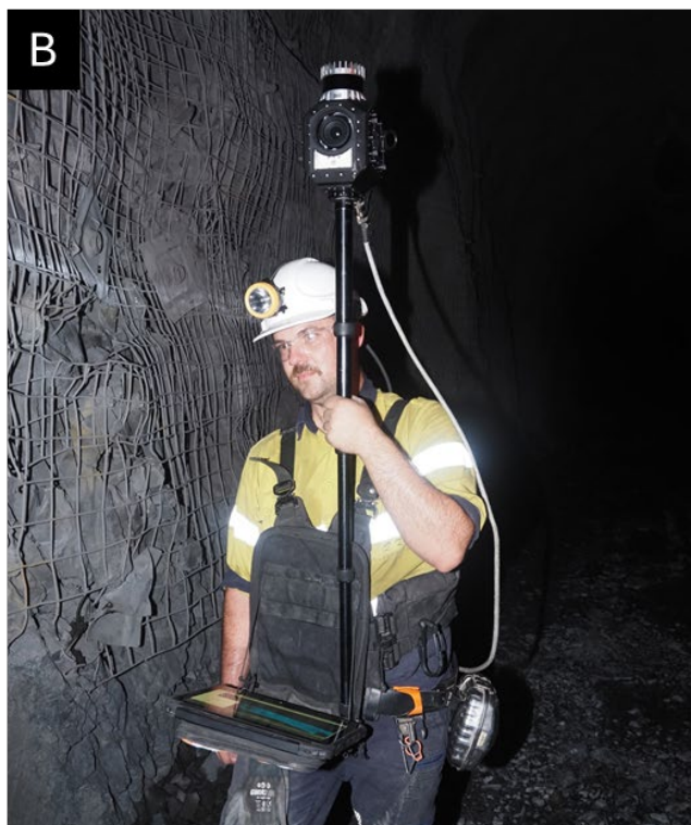
FIG 2 – Top (A) The MVS FC Mapping System components; Bottom (B to C) shows the system in use underground.
