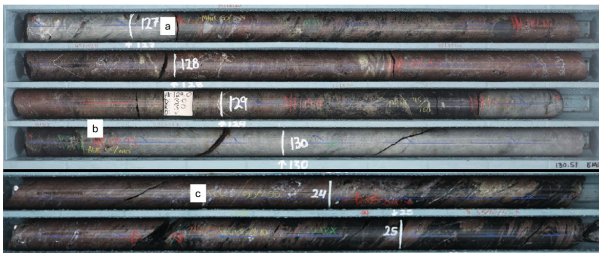
FIG 3 – Photos of drill core with geology mark-up. Examples of mineralisation contacts ('MINC', a), alteration contacts ('ALTC', b) and foliation ('FOL', c) marked in yellow chinagraph on drill core.
