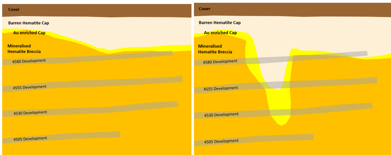
FIG 7 – Left shows original interpretation with surface only data, right image shows interpretation with wall mapping and limited sub-horizontal drilling for these levels.
