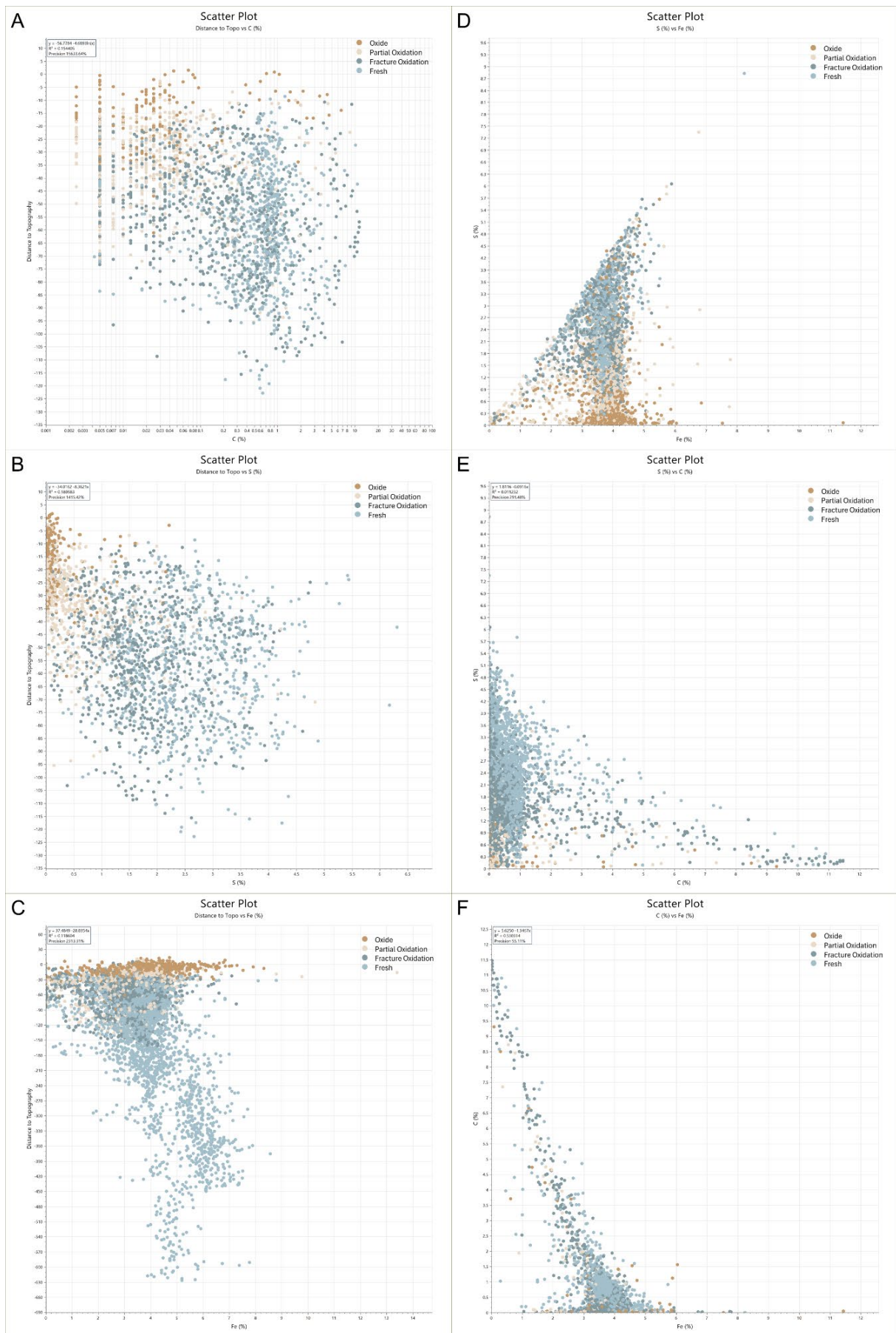
FIG 13 – Scatter plots of distance-to-topography versus C, S and Fe (a to c), and S versus Fe, S versus C and C versus Fe (d to f).
