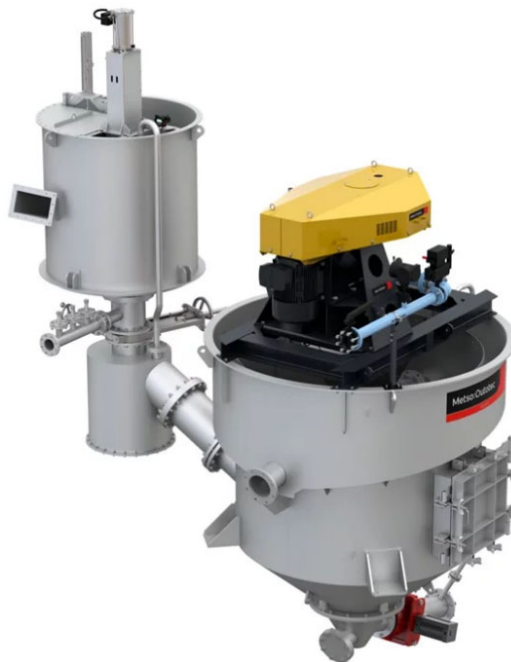
FIG 3 – Metso SkimAir flash flotation cell (Metso.com).
