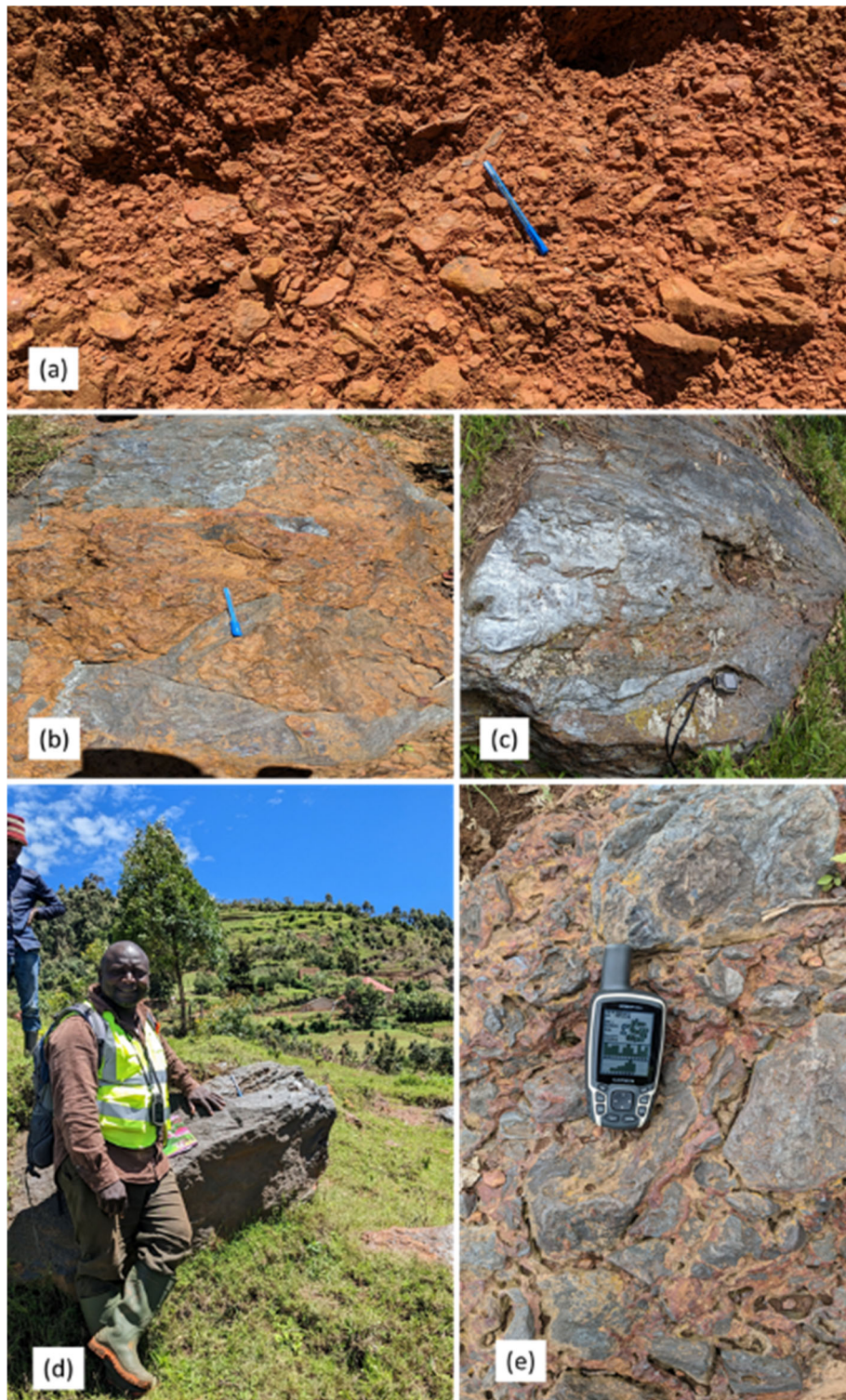
FIG 17 – (a) Scree layer capping massive hematite in north of zone B; (b) goethite coated massive boulders in zone A; (c) massive specularite boulders in zone B; (d) Massive blue Hematite boulder outcrop in zone A; and (e) Fragments of high-grade ore cemented by iron oxides in zone A (Brecciated ore).
