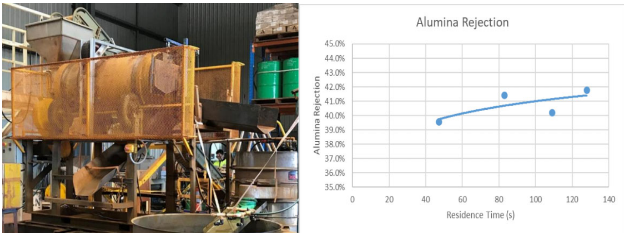
FIG 3 – Pilot drum scrubbing testing arrangement and alumina rejection results.
