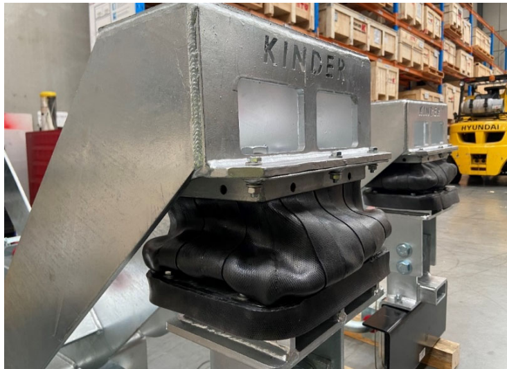
FIG 23 – Torsion spring boot added to prevent ingress.
