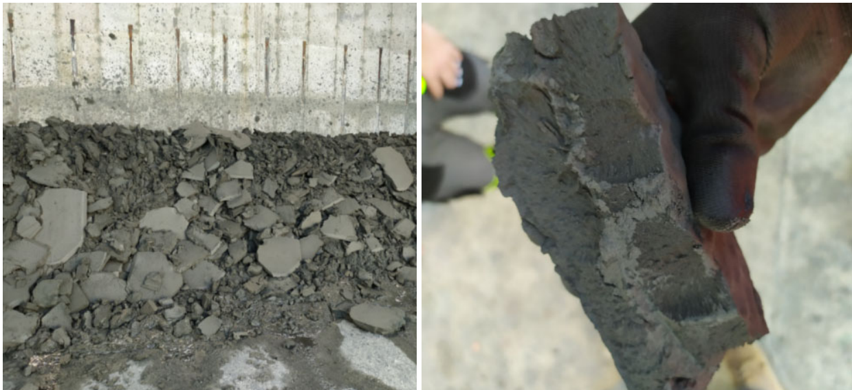
FIG 11 – Cake discharged during commissioning of different tailings plant.
