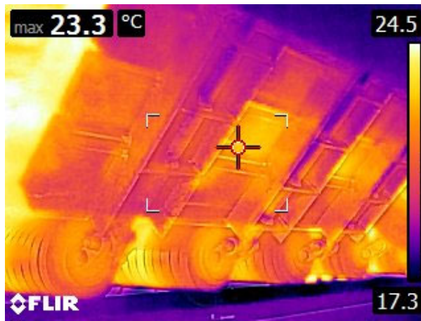
FIG 17 – Temperature data showed it was unlikely to exceed the allowable for the K-Glideshield® material.
