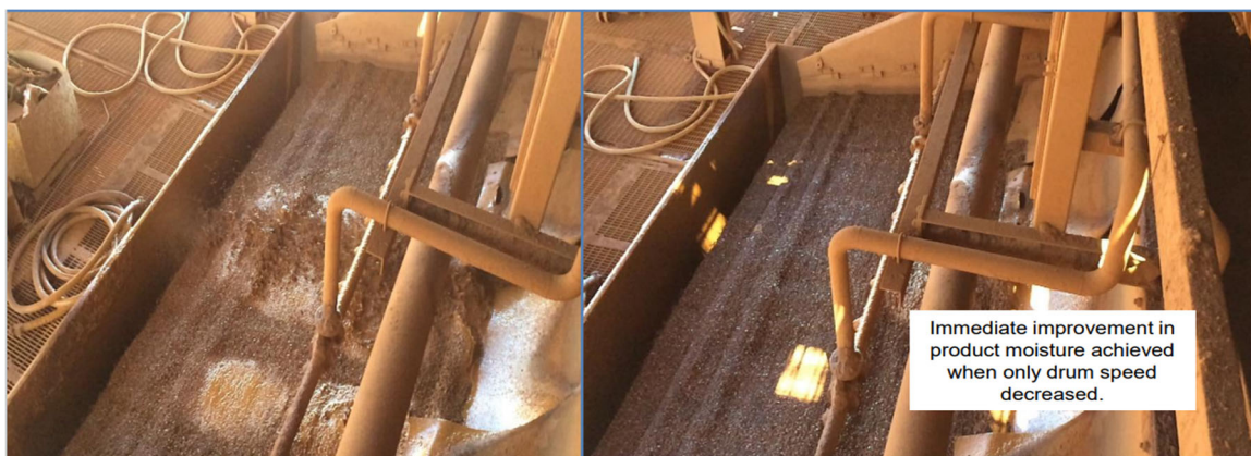
FIG 9 – Improvement in wet screen operation following a reduction in drum speed.
