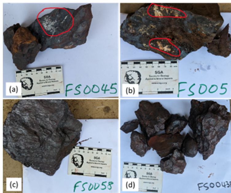
FIG 22 – (a) high-grade hematite sample with quartz; (b) massive ore with pockets of quartz; (c) massive blue hematite; and (d) botryoidal hematite indication iron remobilisation.
