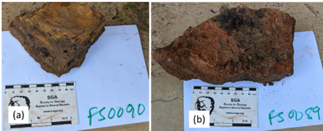
FIG 27 – Goethite samples from Rwengongo with: (a) yellowish brown stained by goethite ore; and (b) vuggy nature as a result of quartz leaching.
