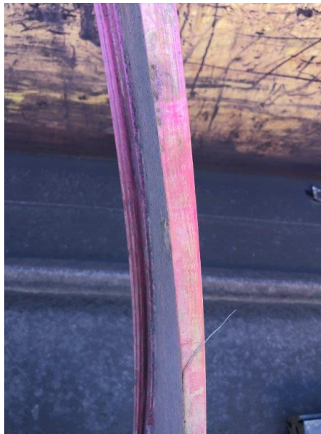
FIG 14 – Variable wear thickness along slider rail.
