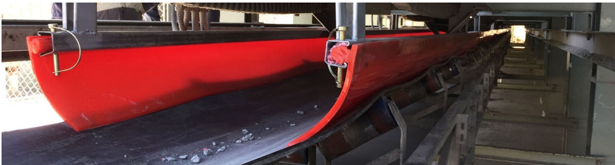
FIG 21 – K-Snap Loc® lay in belt skirting system can self-adjust to belt sag and skirting wear.
