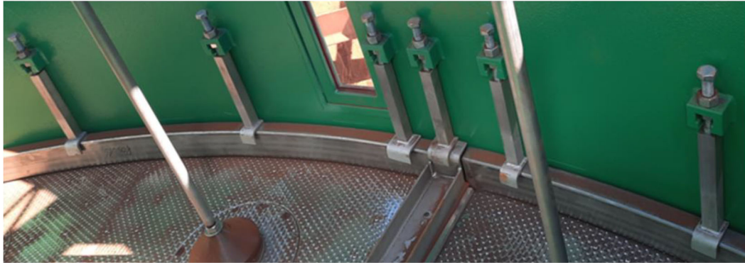
FIG 9 – New fix arrangement for conidur plates.
