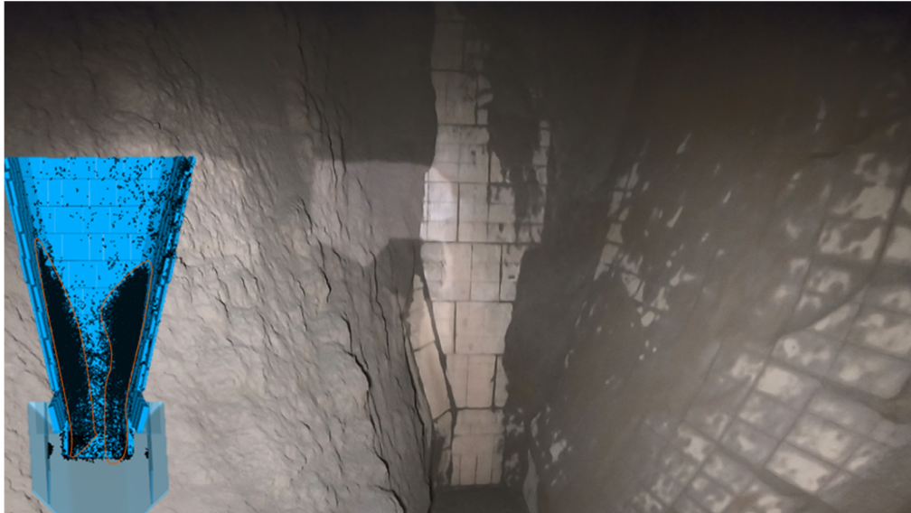
FIG 7 – Material build-up pattern compared to DEM build-up. As shown, close agreement between the DEM simulation and real-life wear pattern was achieved with proper calibration of the DEM adhesive and cohesive properties.
