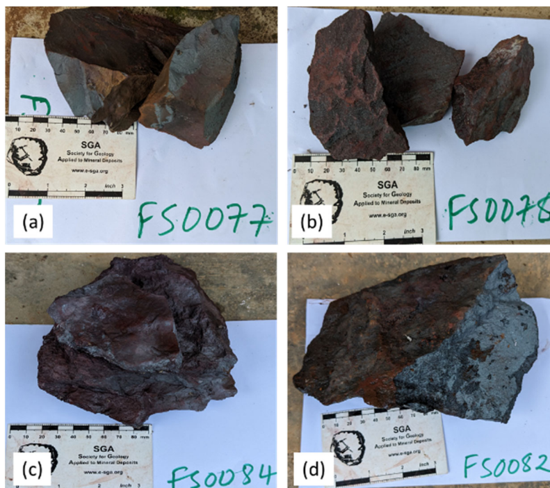
FIG 10 – (a) Massive blue hematite ore; (b) microplaty hematite sample; (c) specularite sample; and (d) massive vuggy bluish hematite.
