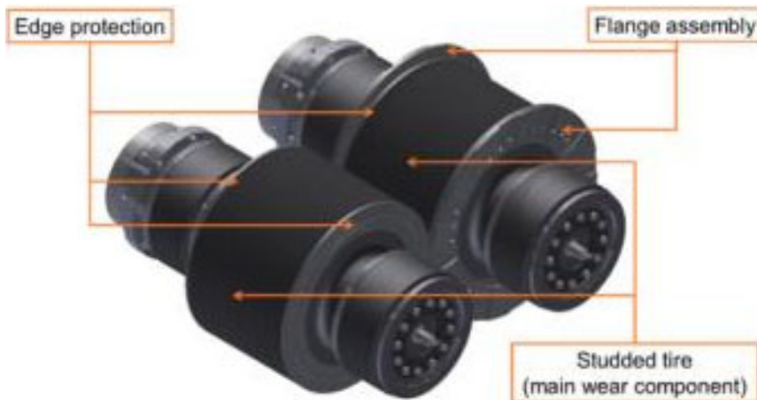
FIG 4 – HRC™ HPGR flanged rolls.
