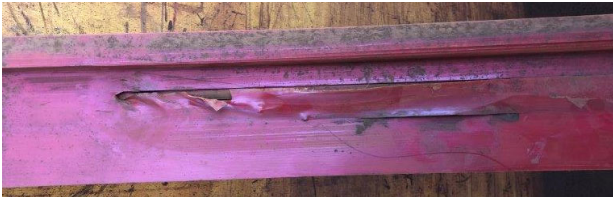
FIG 15 – Signs of friction generated burning on the slider rail.
