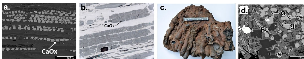
FIG 1 – (a) SEM backscattered electron image, (b) Optical micrograph showing high calcium oxalate (CaOx) crystal development in Syzygium Zeylanicum , (c) image of slag iron sample, (d) BSE image showing slag iron mineralogy.
