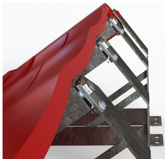
FIG 13 – Possible failure mode under high ambient temperature or high belt speed and capacity conditions, placing higher loads on smaller areas due to sagged slider rails once the softening temperature is reached.
