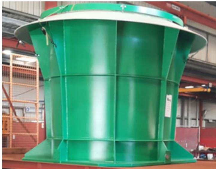
FIG 5 – Rotable Coarse Section at the workshop.
