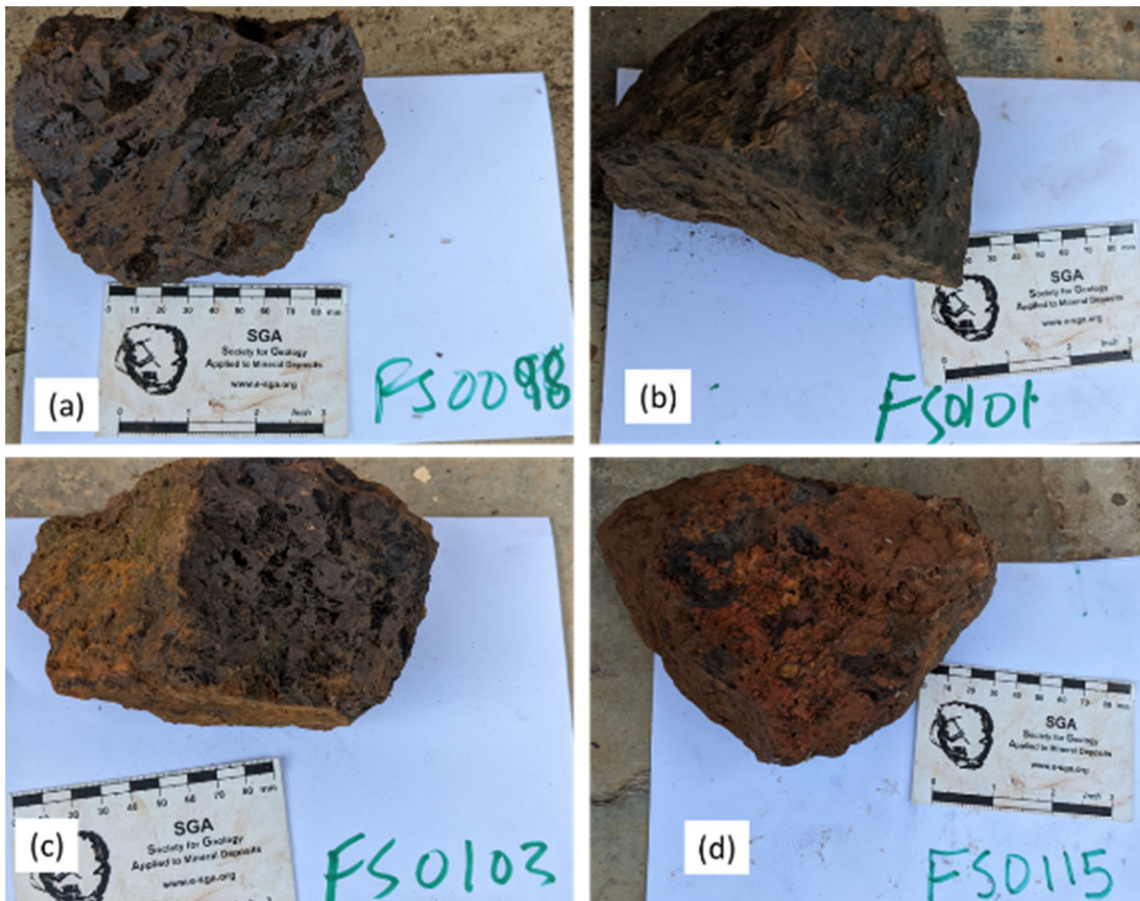
FIG 29 – Goethite samples showing dark brown colours with dark spots (a and c) and earthy colours with vuggy textures (b and d).
