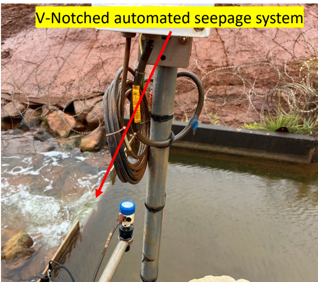
FIG 3 – Automated seepage system (left) versus manual method (right).
