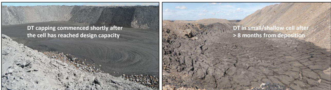
FIG 2 – Dewatered tailings (DT) disposed in cells with different desiccation periods.
