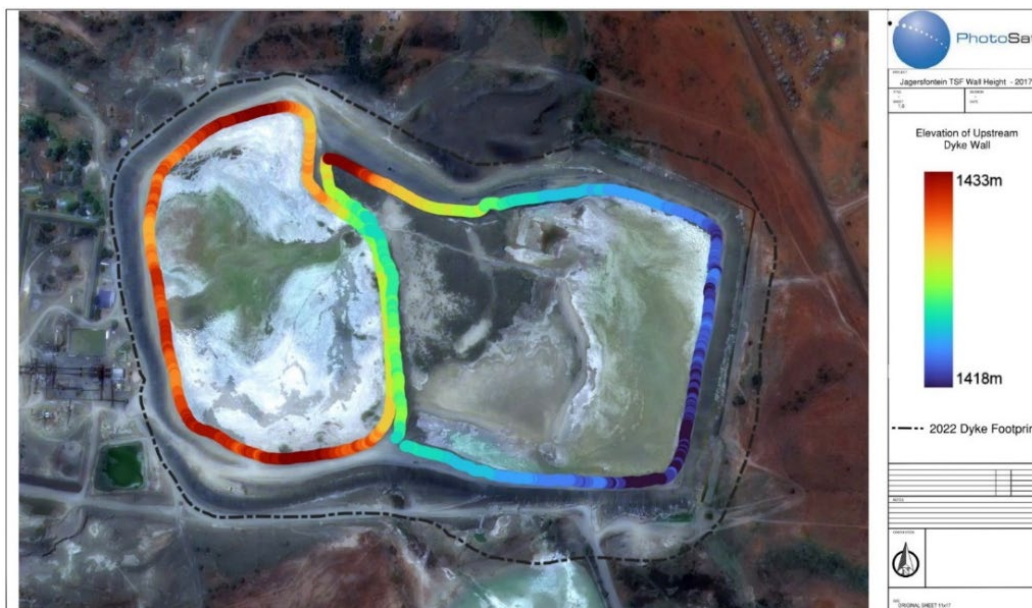
FIG 24 – Dam crest height for 2017.
