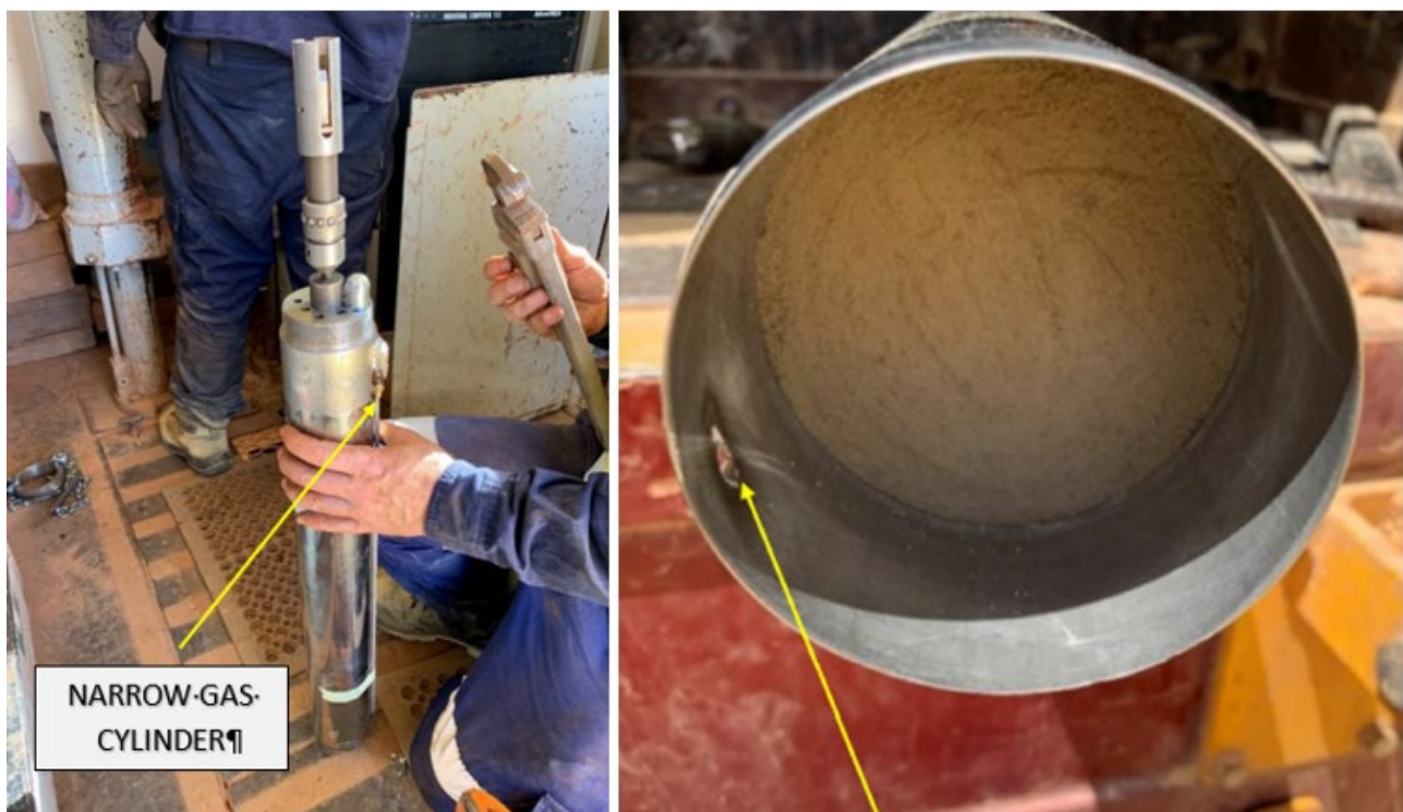
FIG 1 – Tube sampler showing gas cylinder (left) and tube cutting face (right) showing CO 2 injection hole and squared off sample.
