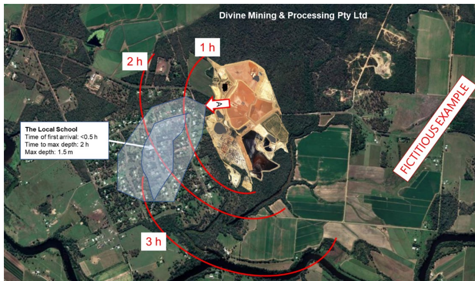
FIG 4 – Individual inundation map with points of interest and isochrones, showing estimated time of arrival. Fictitious example.
