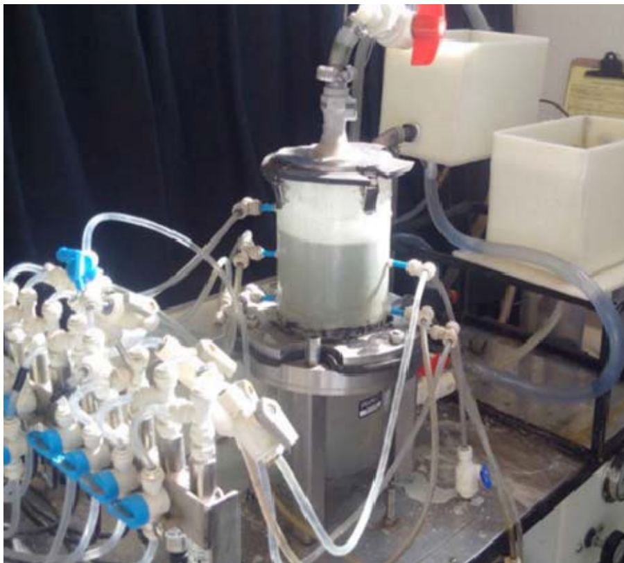
FIG 8 – Set-up of the filtration test (Gradient Ratio test, ASTM D5101).
