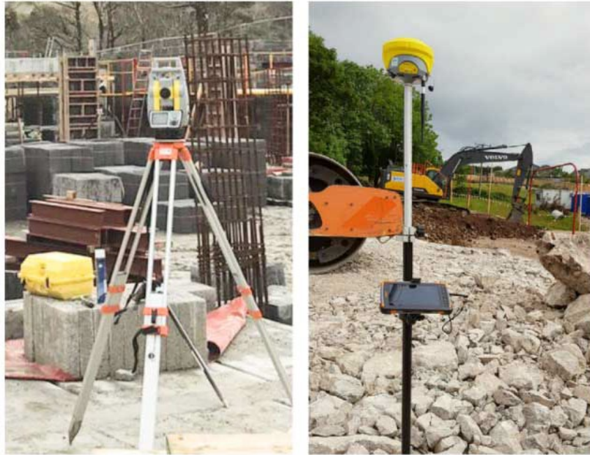
FIG 1 – Photographs of total station and GPS rover (source: Hanrahan and Hanmore, 2021).
