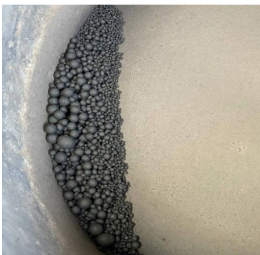
FIG 5 – Produced CTBAs using disc pelletiser.
