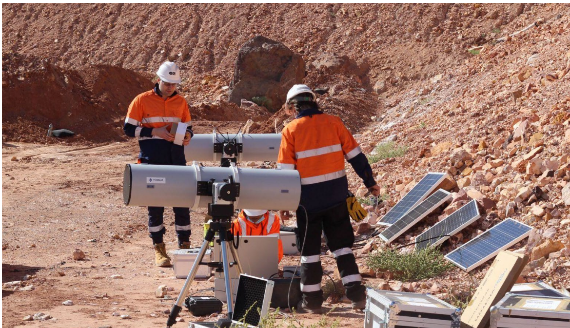
FIG 2 – Top, showing a qualitative sketch representing, left, optically isolated scintillation slabs and, right, which allow for a geometric reconstruction of a muon trajectory (indicated by a star/red line). Bottom, two telescopes mid-installation (note not their final placements), with reference muon counter as the small black box at its base.
