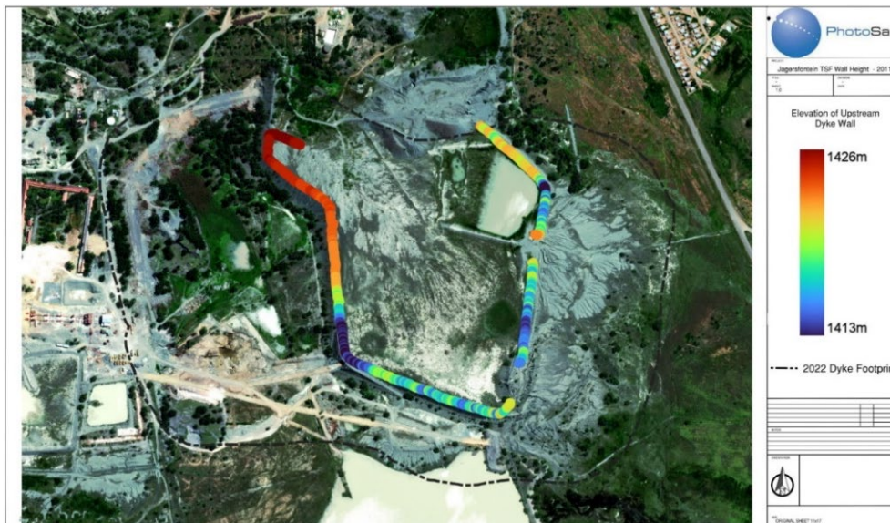
FIG 23 – Dam crest height for 2011.
