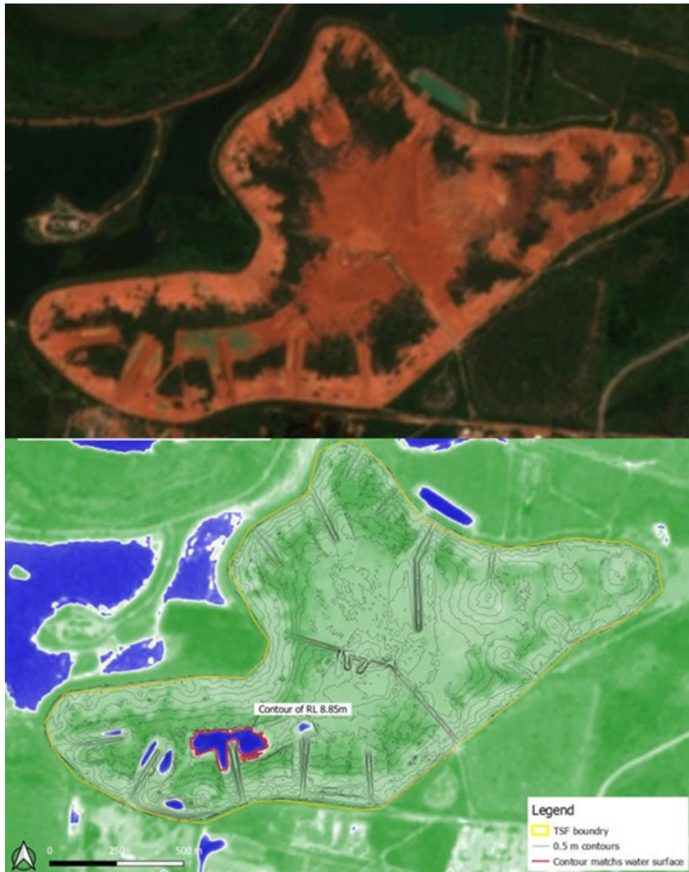
FIG 3 – Sentinel-2 Images – True Colour (upper image) and NDWI (lower image, blue is water surface estimate) used to calculate water levels.
