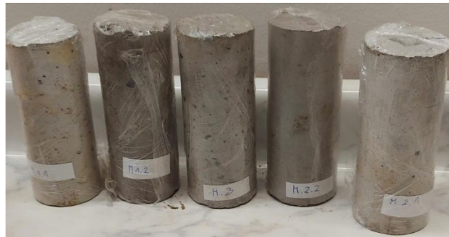
FIG 12 – Samples of consolidated polymers.
