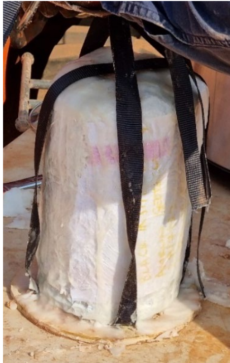
FIG 13 – Mini-block sample coated in wax and aluminium foil, located on custom-made base.
