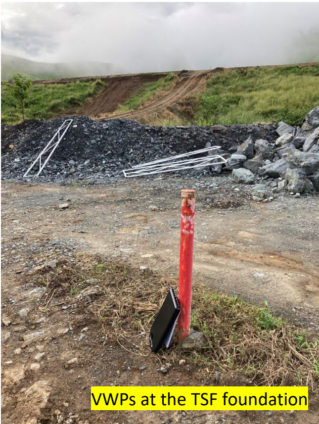
FIG 2 – Installed online stream monitoring systems at the TSF Foundation (left) and dam crest (right).
