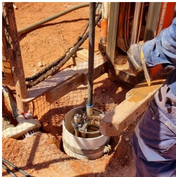
FIG 12 – Mini-block sampler being lowered into the case borehole.
