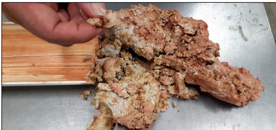
FIG 3 – Voided Bulimba layer broken down and examined.
