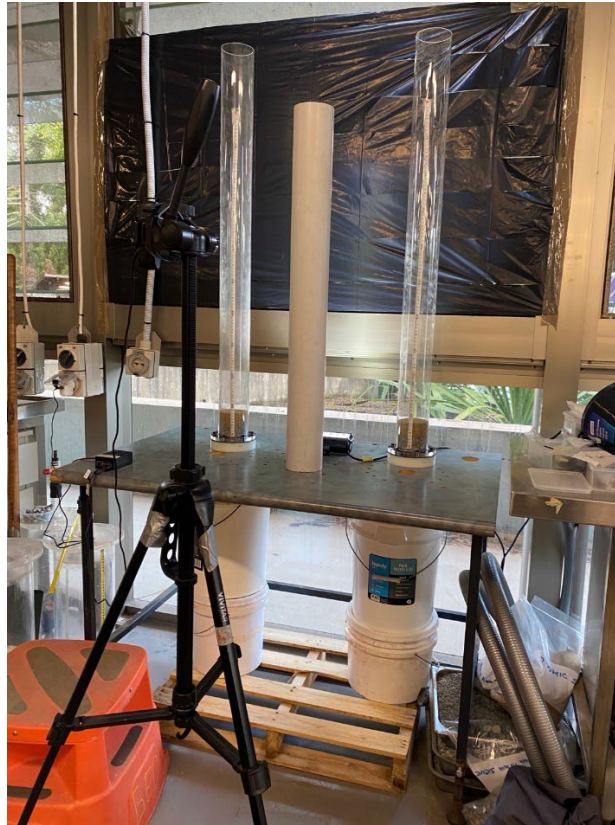
FIG 3 – Leachate column set-up.
