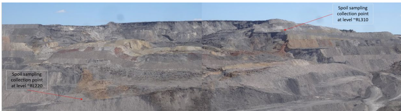
FIG 13 – Approximate location of spoil sample collection locations at levels ~RL220 and ~RL310.
