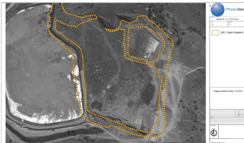
FIG 15 – 2011 Dyke footprint overlaid over October 1st 2014 WV-2 satellite image.
