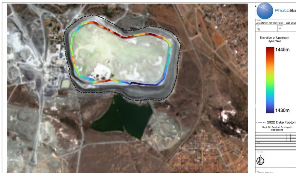
FIG 25 – Dam crest height for 2022 pre-failure.
