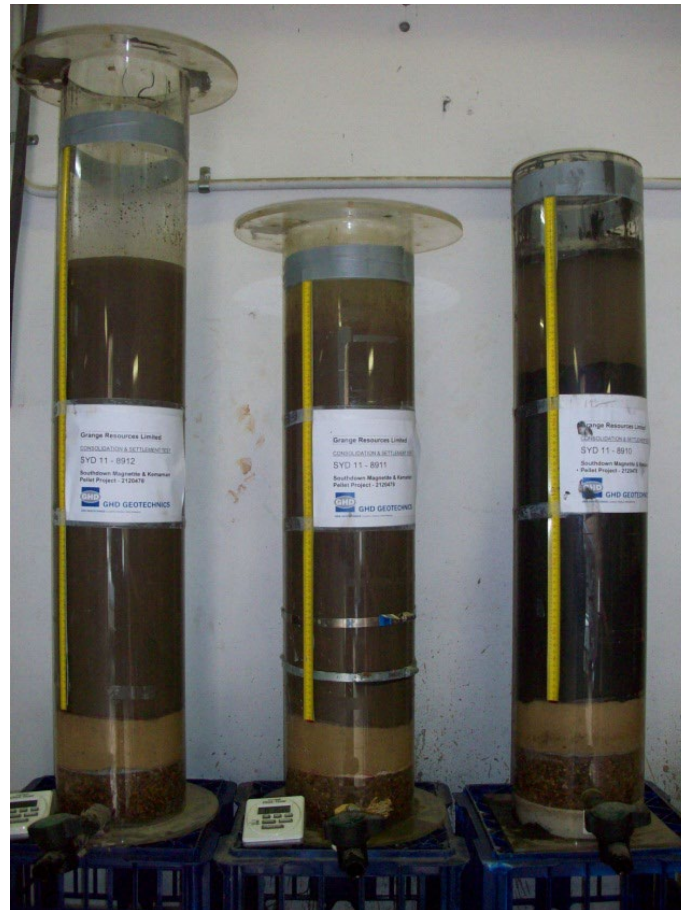
FIG 1 – Column settlement and consolidation test.
