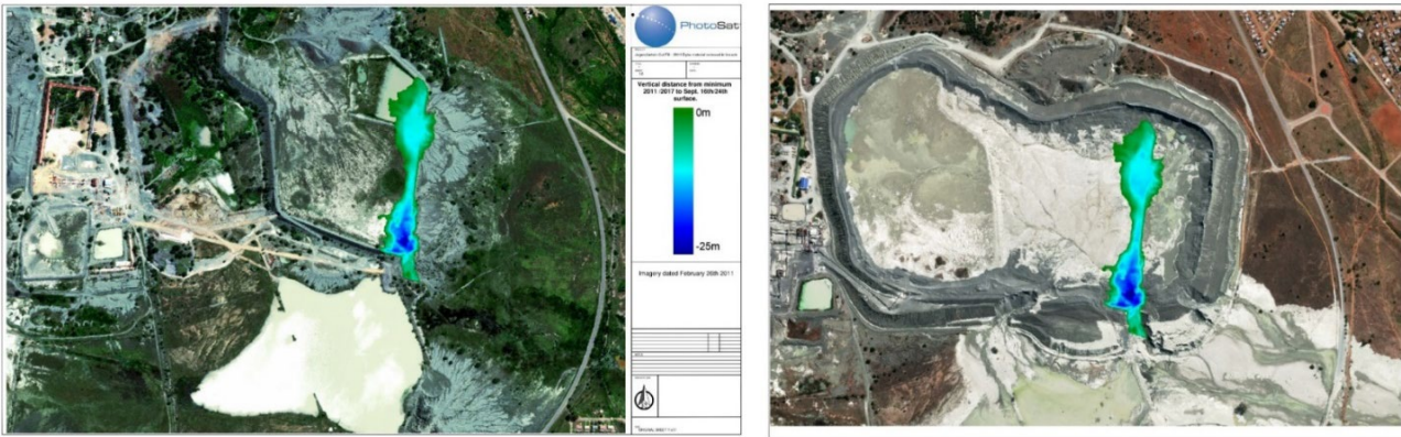
FIG 13 – Cut map overlaid on 2011 and 2022 post-failure orthophoto.
