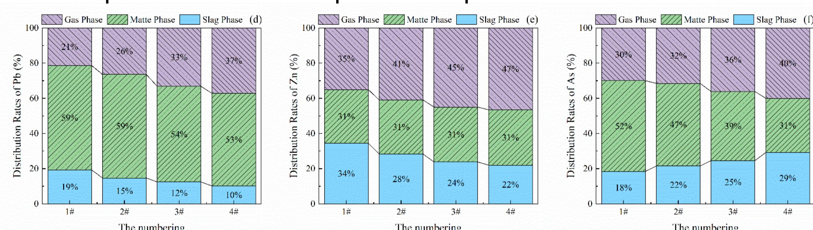
The primary forms of Pb in nickel slag include metallic lead, lead silicate, and lead sulfate. Adjusting slag's composition enhances the stability of Pb compounds in the slag, and reducing the risk of Pb release, while the content of lead iron sulfate gradually increases. When the slag has higher alkalinity, CaO more easily combines with silicate ions, displacing Fe and resulting in lower lead silicate content and higher lead iron sulfate content in the slag.
