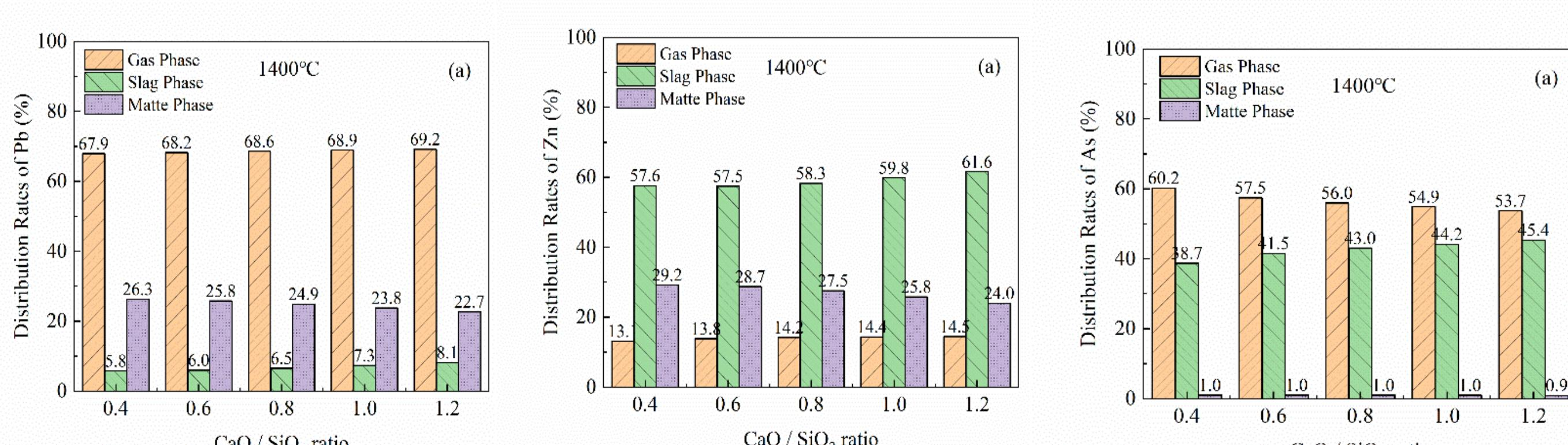
As the content of CaO in the slag increases, the content of Pb, Zn, and As in the gas and matte increases and decreases, respectively. The content of Pb, Zn in the slag decreases, while the content of As in the slag increases. The deviation between test results and theoretical calculations is attributed to the difference between equilibrium state and the nonequilibrium state in experimental processes.
