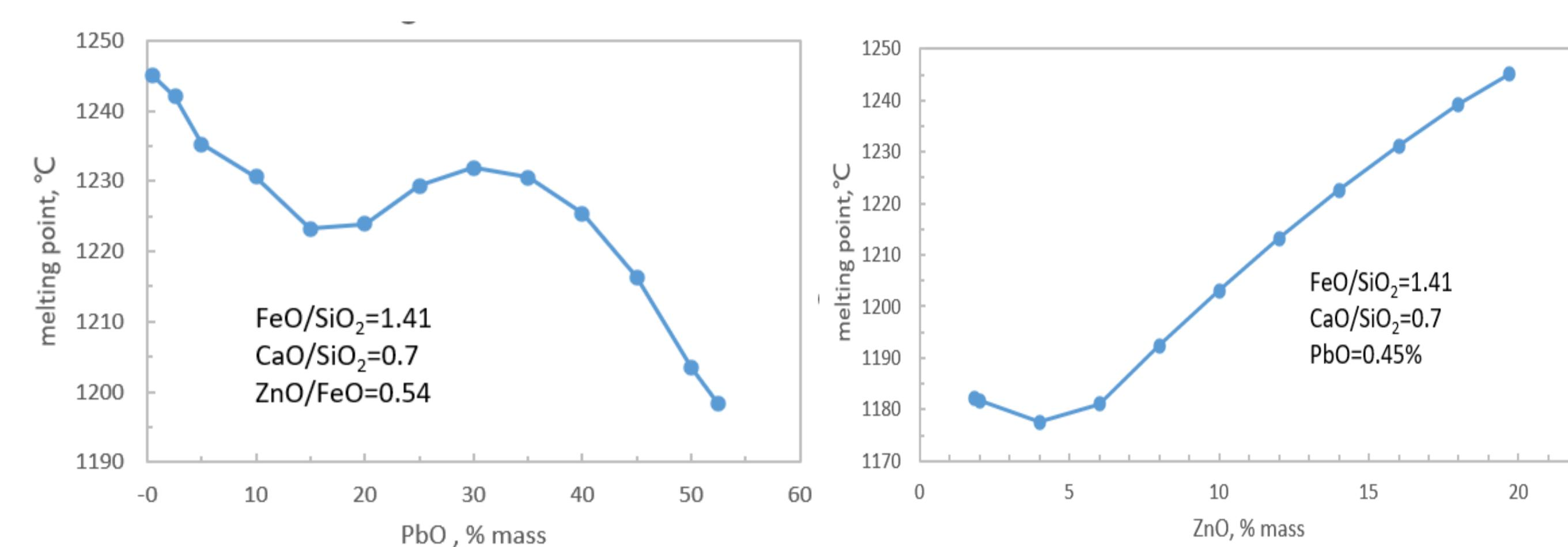
The test results is in accordance with these. With the PbO content decreased from 43.09% to 2.69%, the melting point increased from 1158°C to 1269°C. The viscosity also increased to some extent.
