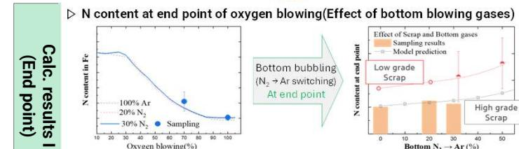
As is: Quantification of N content by %N<sub>2</sub> B.B. (N<sub>2</sub> B.B. after 50%: acceleration of N pick-up)
