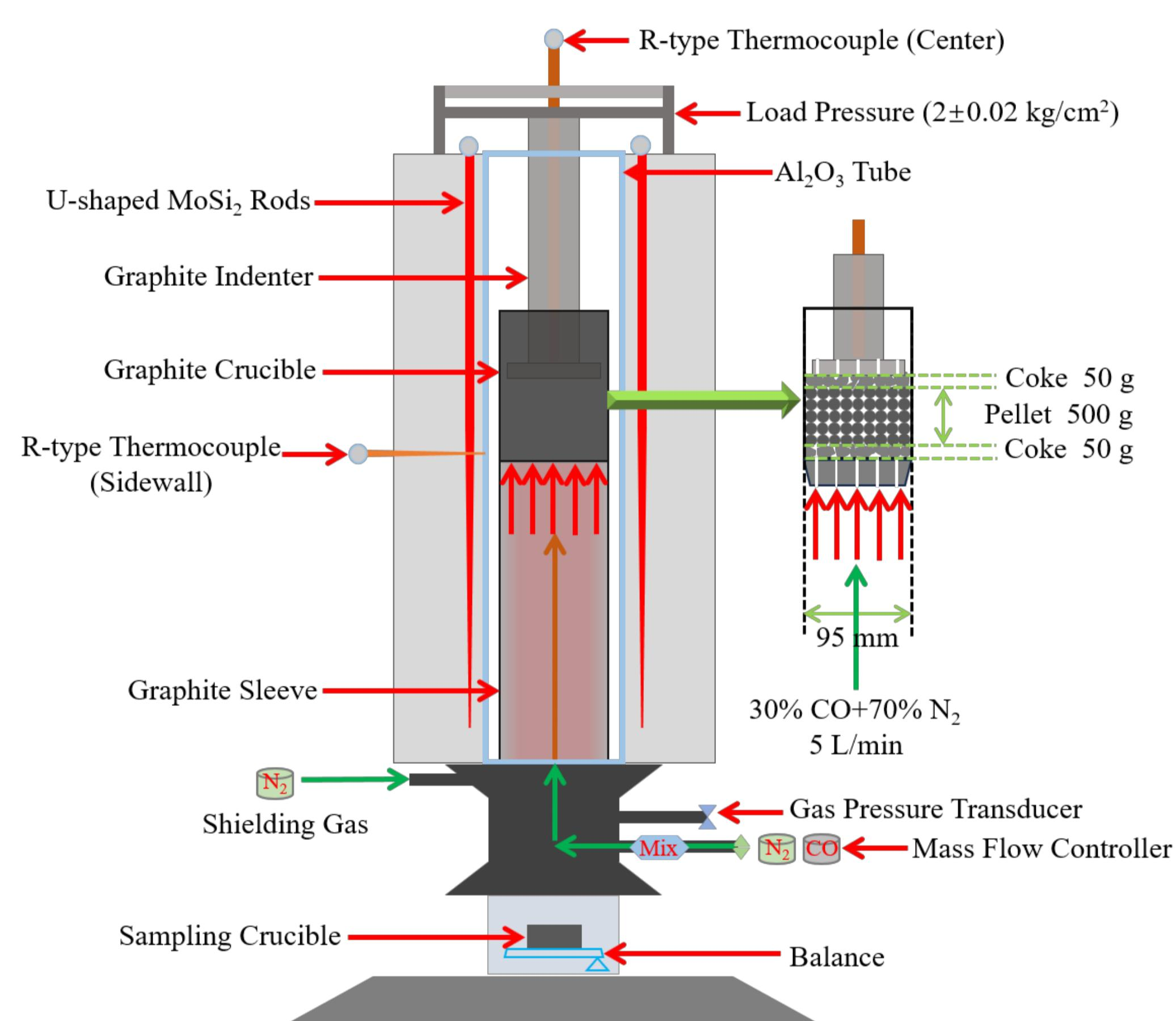
The titanium-bearing burden used in the experiments were acid and fluxed pellets (basic pellets) prepared from Sea Sand Vanadium Titanomagnetite (SSVTM), Low Chromium-bearing Vanadium Titanomagnetite (LCVTM), and High Chromium-bearing Vanadium Titanomagnetite (HCVTM), respectively. The softening-melting properties of the above pellets were carried out in the high-temperature softening-melting-dripping properties test furnace.
