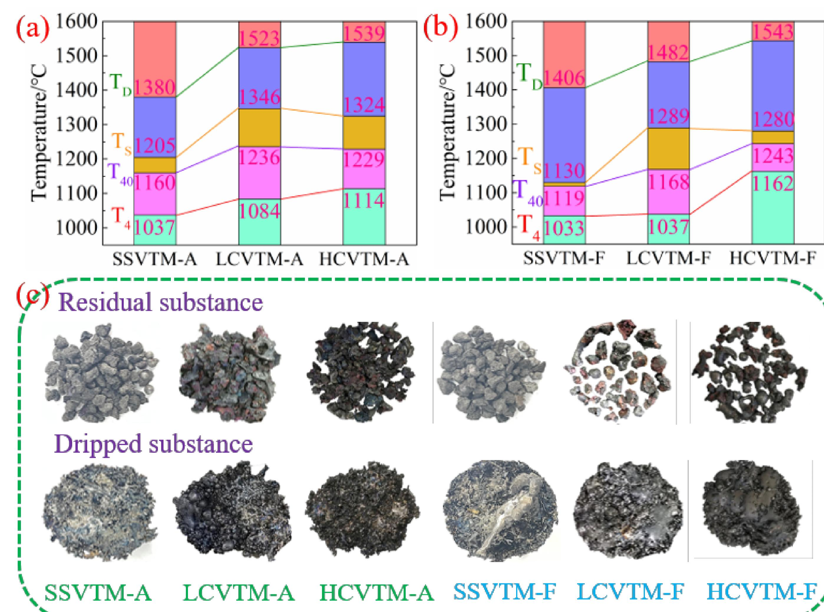
Compared with the softening-melting performance of SSVTM-A, the softening start and softening end temperatures of LCVTM-A and HCVTM-A were significantly increased, while the softening intervals became wider and then narrower. The softening-melting intervals  $[T_D-T_4]$  of LCVTM-A and HCVTM-A were significantly wider than those of SSVTM-A, which indicated the deterioration of softening-melting performance indexes.
