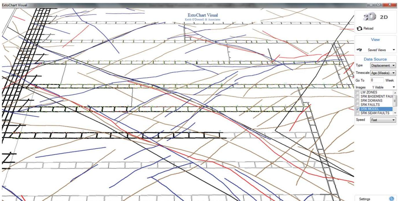
FIG 8 – Springvale mine workings with fault interpretation model.
