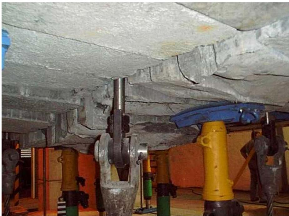
FIG 6 - Discontinuous failure in the stope roof in a test
