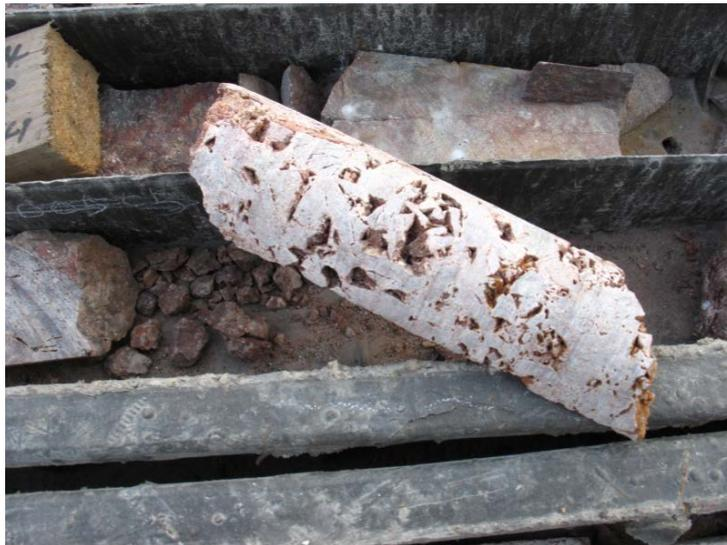
FIG 3 – Examples of potential water bearing zones in drill core
