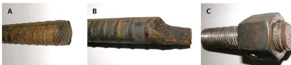
**FIG 1** – (A) Rebar stress corrosion cracking; (B) localised pitting corrosion; (C) thread stress corrosion cracking.
