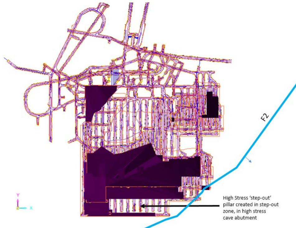
FIG 10: Stepping out into abutment, then mining transverse back towards cave, creating high stress diminishing pillar.
