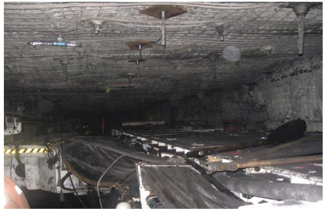
**FIG 14** – Photograph from the main gate corner of the longwall face (looking outbye) in good strata conditions. Note the flat roof and clearance above the main gate longwall equipment.
