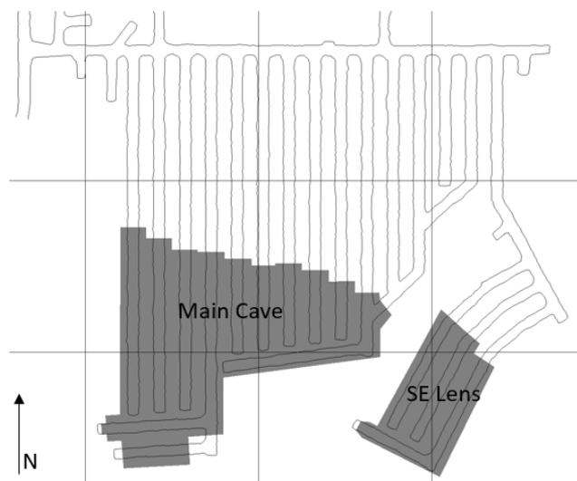
FIG 29: Main cave and Southeast lens advanced in sequence, with the SE lens leadings slightly
