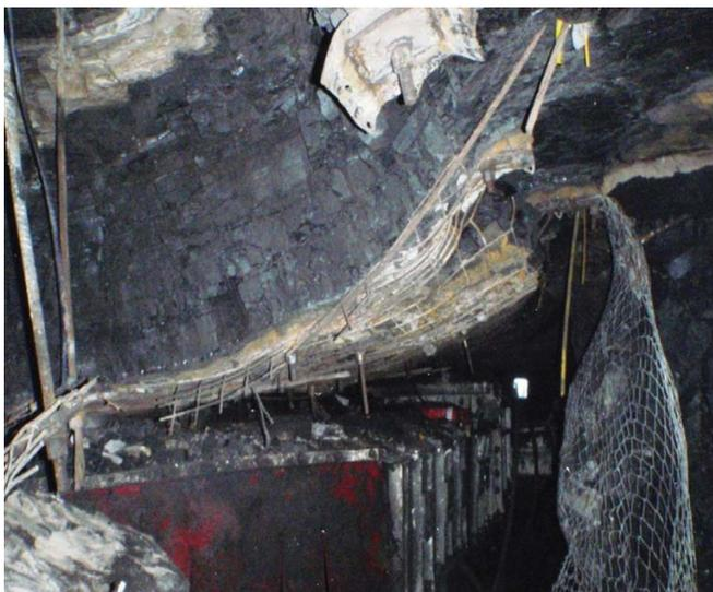
**FIG 16** – Photograph from the main gate corner of the longwall face (looking outbye) in very poor strata conditions. Note the severely deformed roof and lack of clearance above the main gate longwall equipment.
