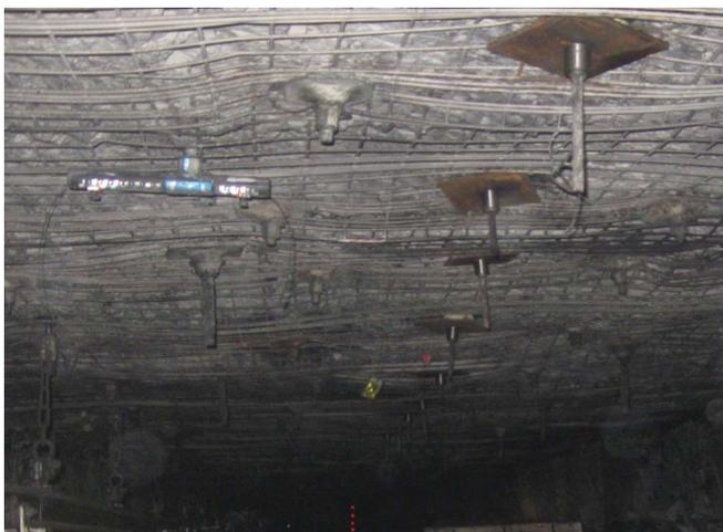
FIG 6 – Telltale installation in underground roadway.
