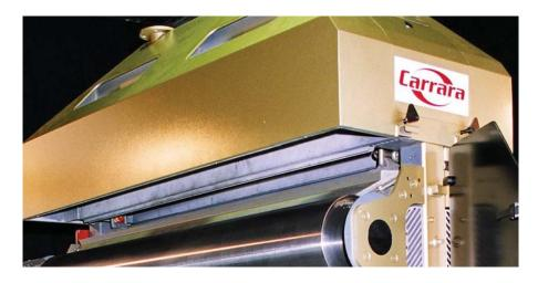
Electrostatic separators are used to separate dry, free flowing materials with particles sizes between 40 and 800 microns that exhibit electrical conductivity differences.
