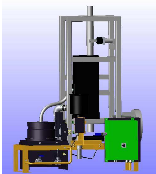
Figure 14. The flexible hose sampler followed by a one pot vacuum drying unit.
