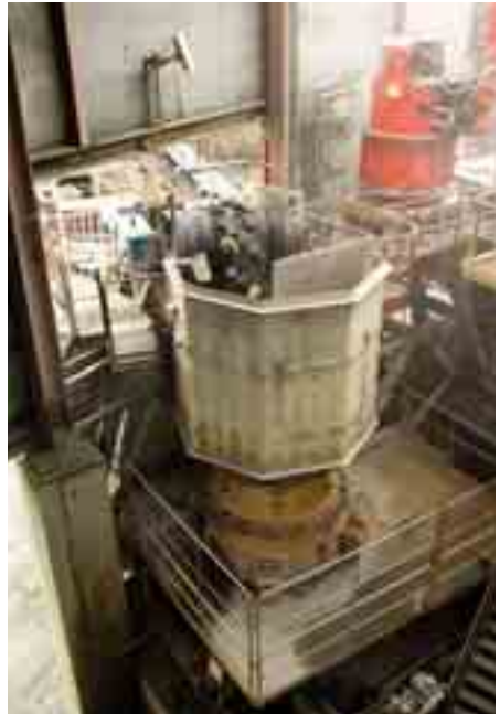
2. Nordberg GP500S operating as a secondary crusher following C160 primary crusher
