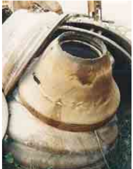
Example of excessive liner use
