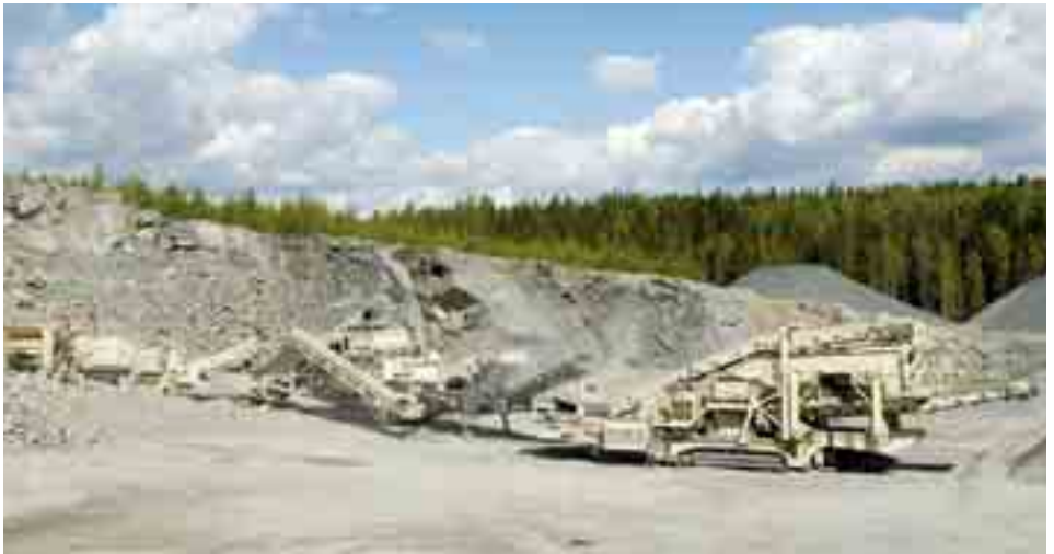
3. Track mounted three stage crushing plant with secondary and tertiary GP-cones
