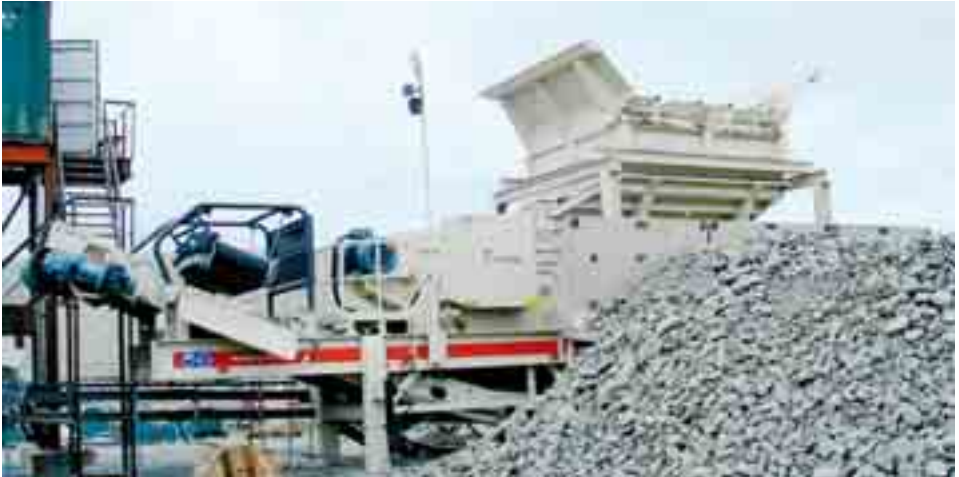
NW106 with primary grizzly on the feed hopper. To prevent oversize material enter to the crusher. Alternative for the hydraulic rock breaker.
