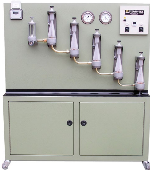
Figure 5. Cyclosizer M14 model with digital flowmeter (Metcon Laboratories, 2008).
