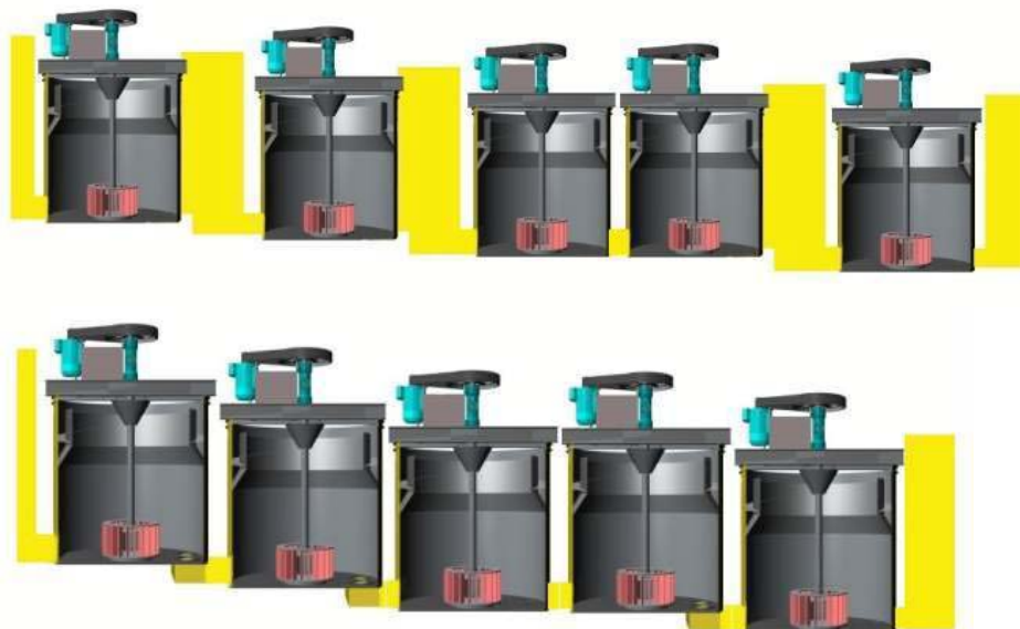
Fig 5: Example flotation bank with external dart valves (Top) and internal dart valves (Bottom)
